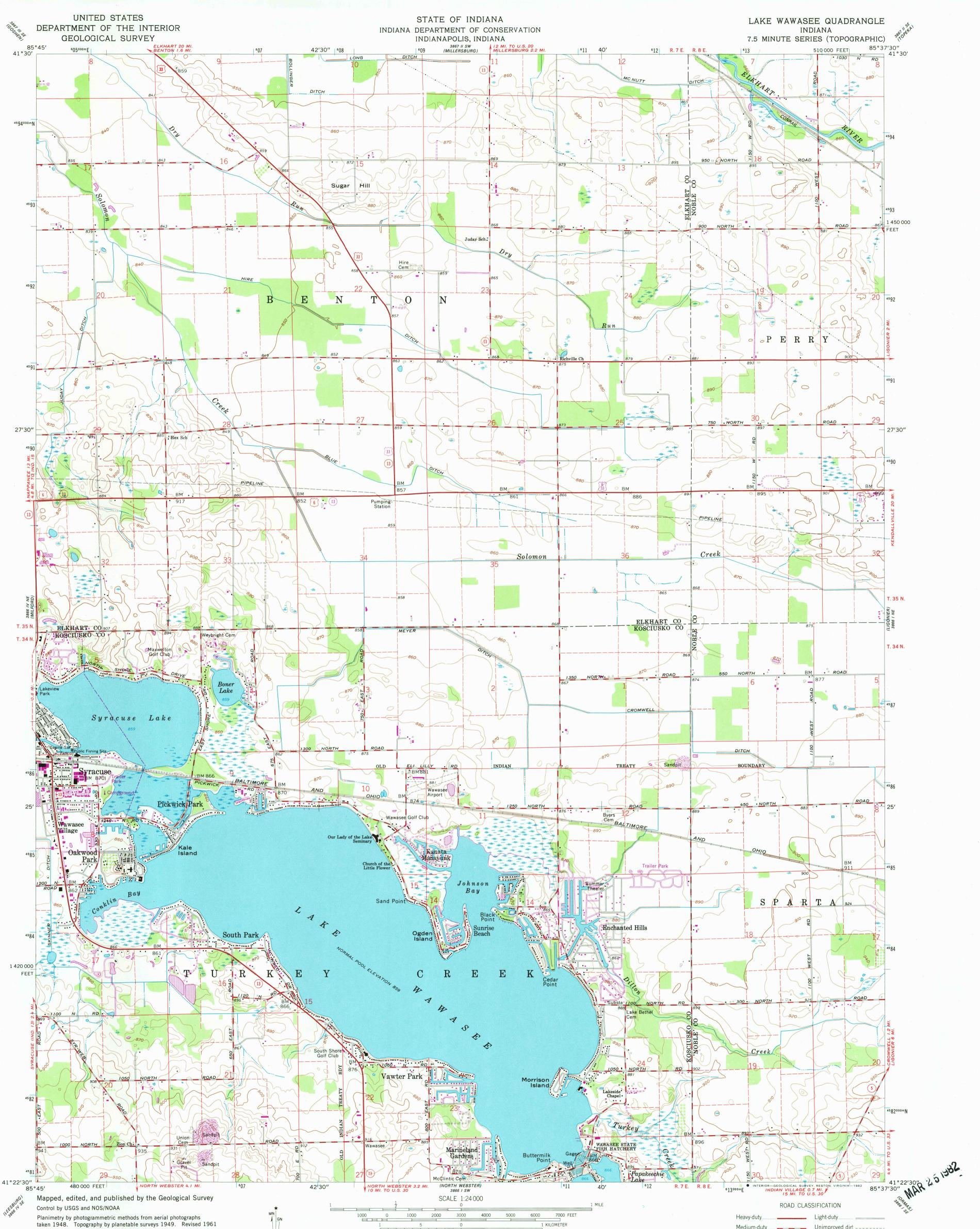
Polyconic projection. 10,000-foot grid ticks based on Indiana coordinate system, east zone. 1000-meter Universal Transverse Mercator grid ticks, zone 16, shown in blue. 1927 North American Datum No adjustment is necessary to place this map on the predicted North American Datum 1983
