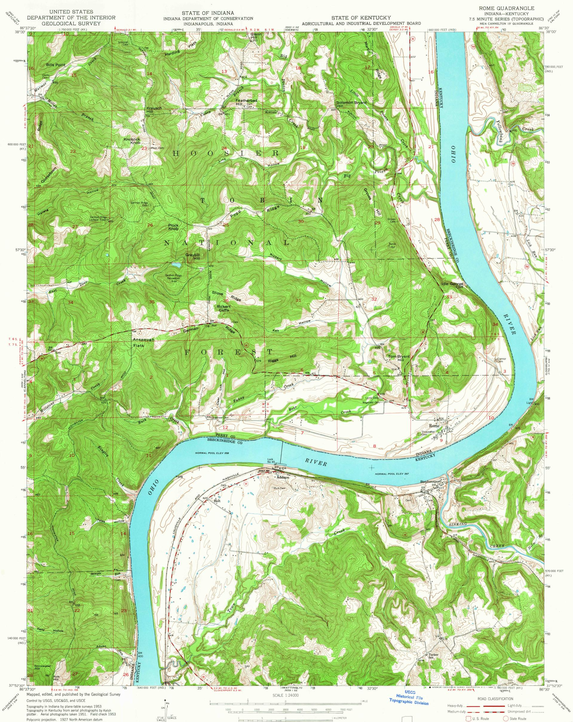
Polyconic projection. 1927 North American datum 10,000-foot grids based on Indiana coordinate system, west zone, and Kentucky coordinate system, south zone 1000-meter Universal Transverse Mercator grid ticks, zone 16, shown in blue
