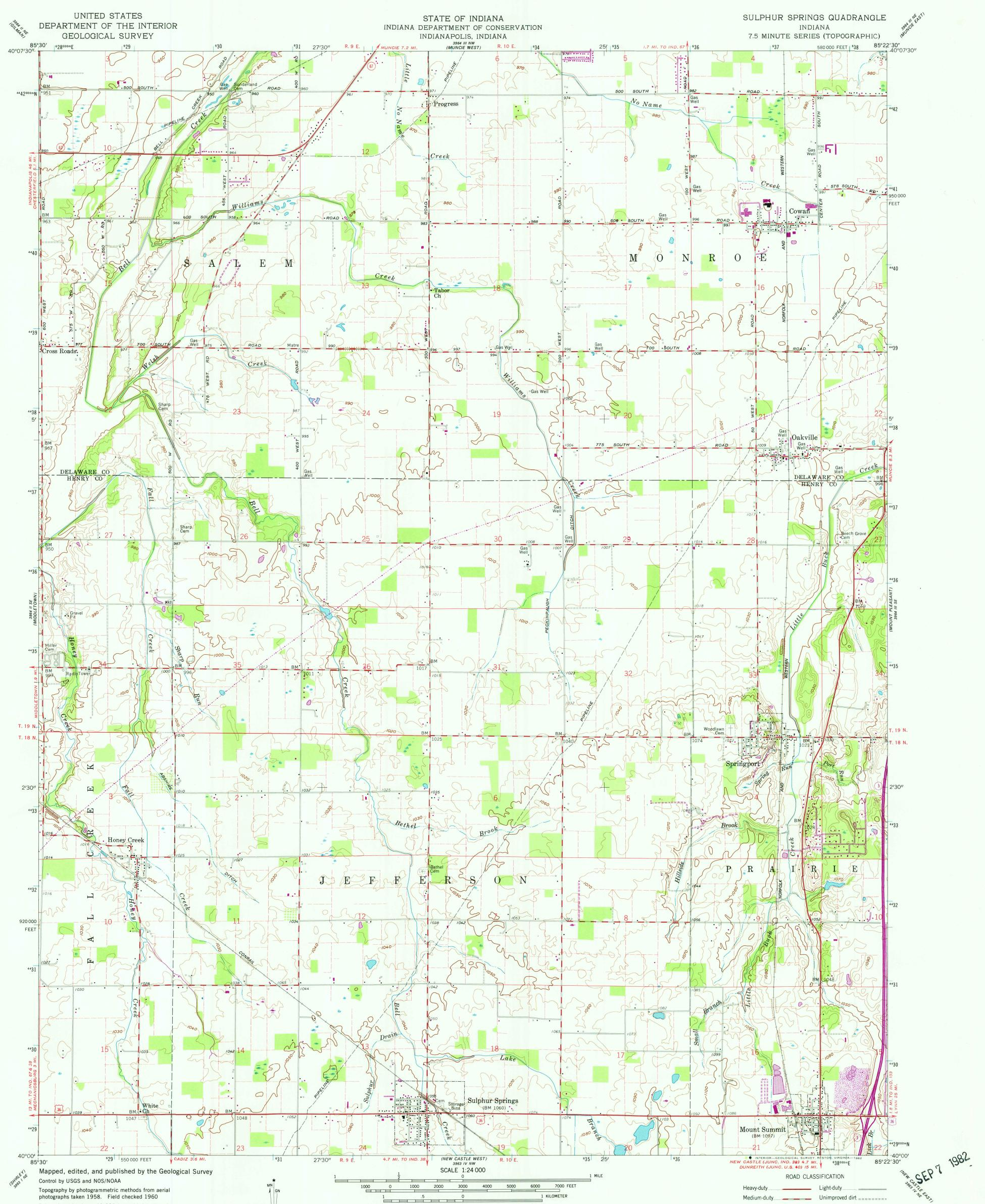
Polyconic projection. 10,000-foot grid ticks based on Indiana coordinate system, east zone 1000-meter Universal Transverse Mercator grid ticks, zone 16, shown in blue. 1927 North American Datum To place on the predicted North American Datum 1983 move the projection lines 1 meter south and 3 meters west as shown by dashed corner ticks
