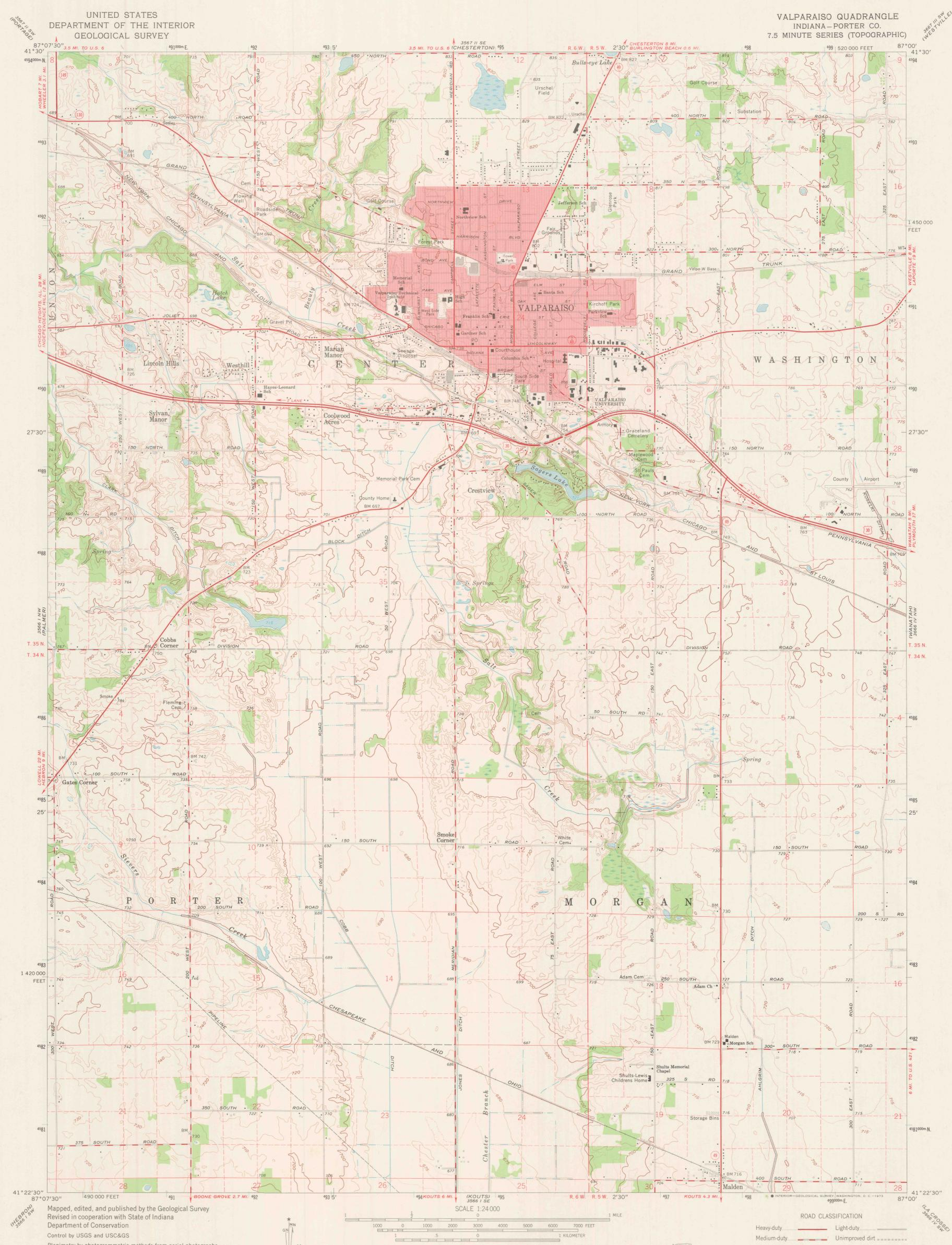
Planimetry by photogrammetric methods from aerial photographs taken 1952. Topography by planetable surveys 1953 Revised 1962
