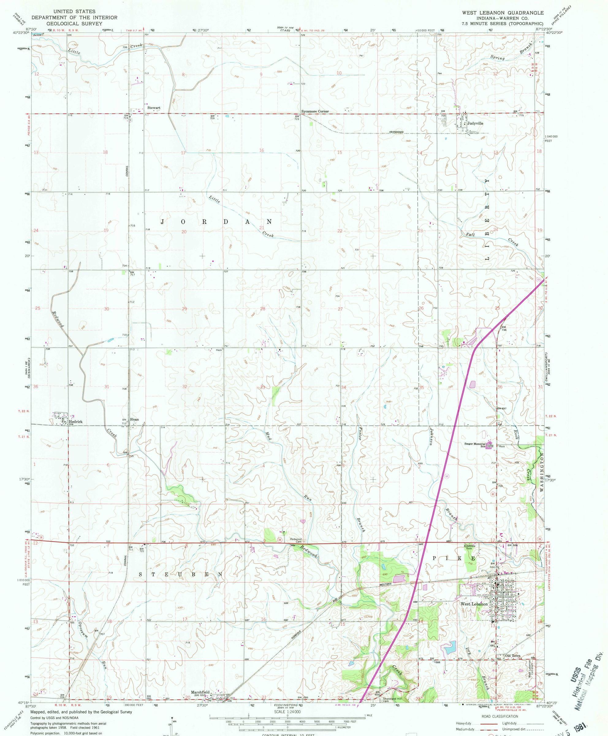
Polyconic projection. 10,000-foot grid based on Indiana coordinate system, west zone 1000-meter Universal Transverse Mercator grid ticks, zone 16, shown in blue. 1927 North American Datum To place on the predicted North American Datum 1983 move the projection lines 3 meters east as shown by dashed corner ticks
