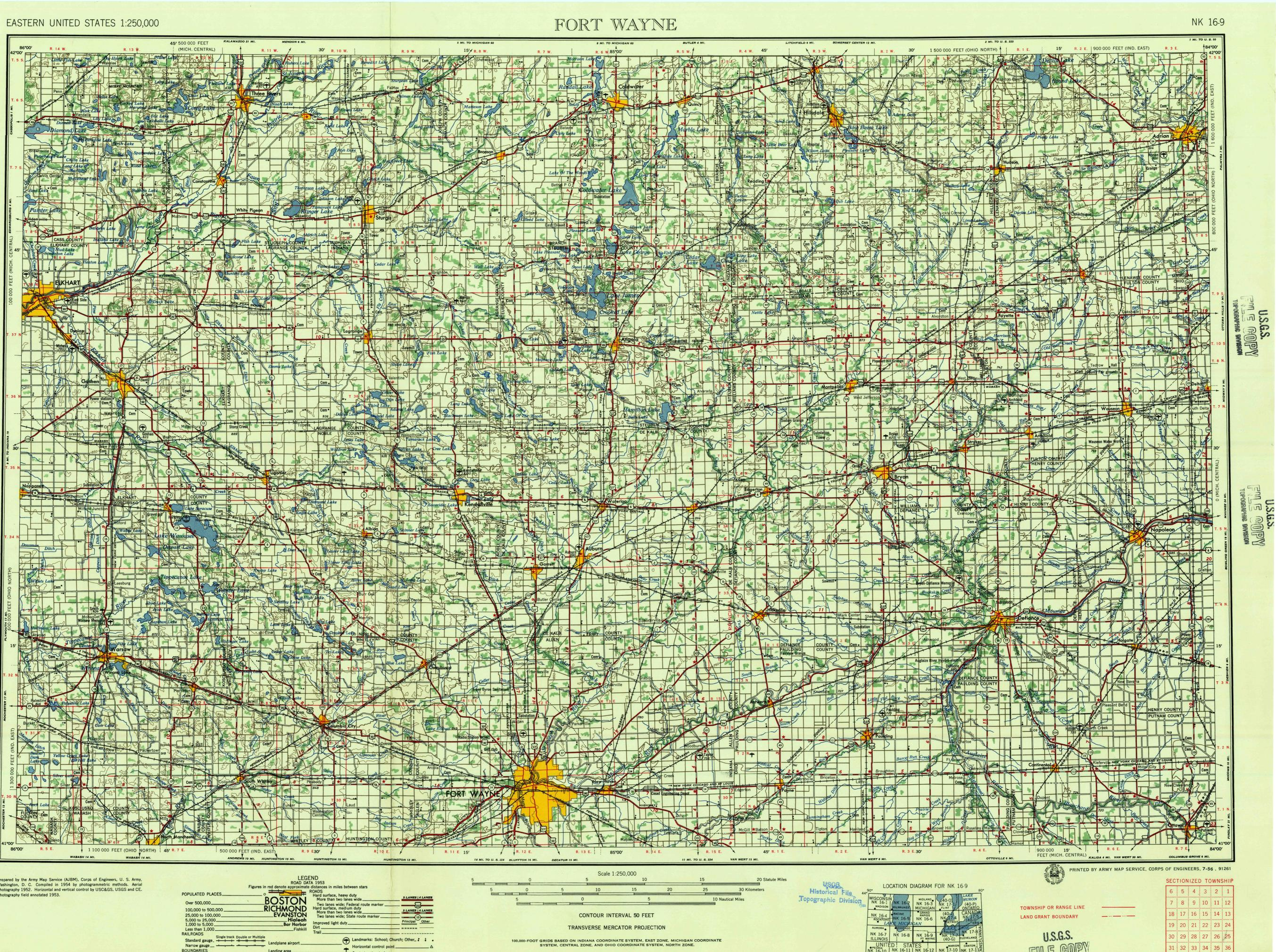
Prepared by the Army Map Service (AJBM), Corps of Engineers, U. S. Army, Washington, D. C. Compiled in 1954 by photogrammetric methods. Aerial photography 1952. Horizontal and vertical control by USC&GS, USGS and CE. Photography field annotated 1953.
