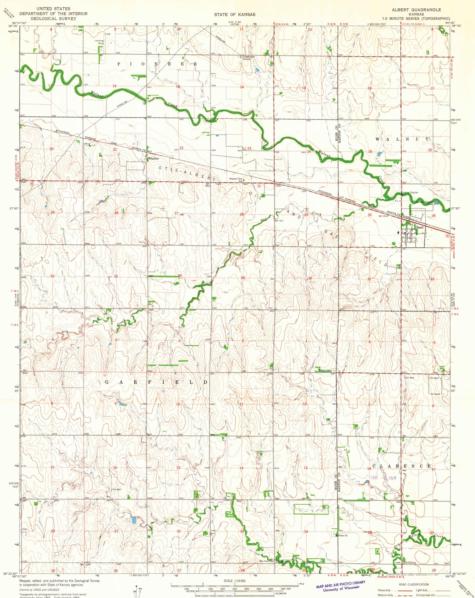
Topography by photogrammetric methods from aerial photographs taken 1964. Field checked 1965 Polyconic projection. 1927 North American datum 10,000-foot grid based on Kansas coordinate system, south zone 1000-meter Universal Transverse Mercator grid ticks, zone 14, shown in blue Fine red dashed lines indicate selected fence and field lines where generally visible on aerial photographs. This information is unchecked
