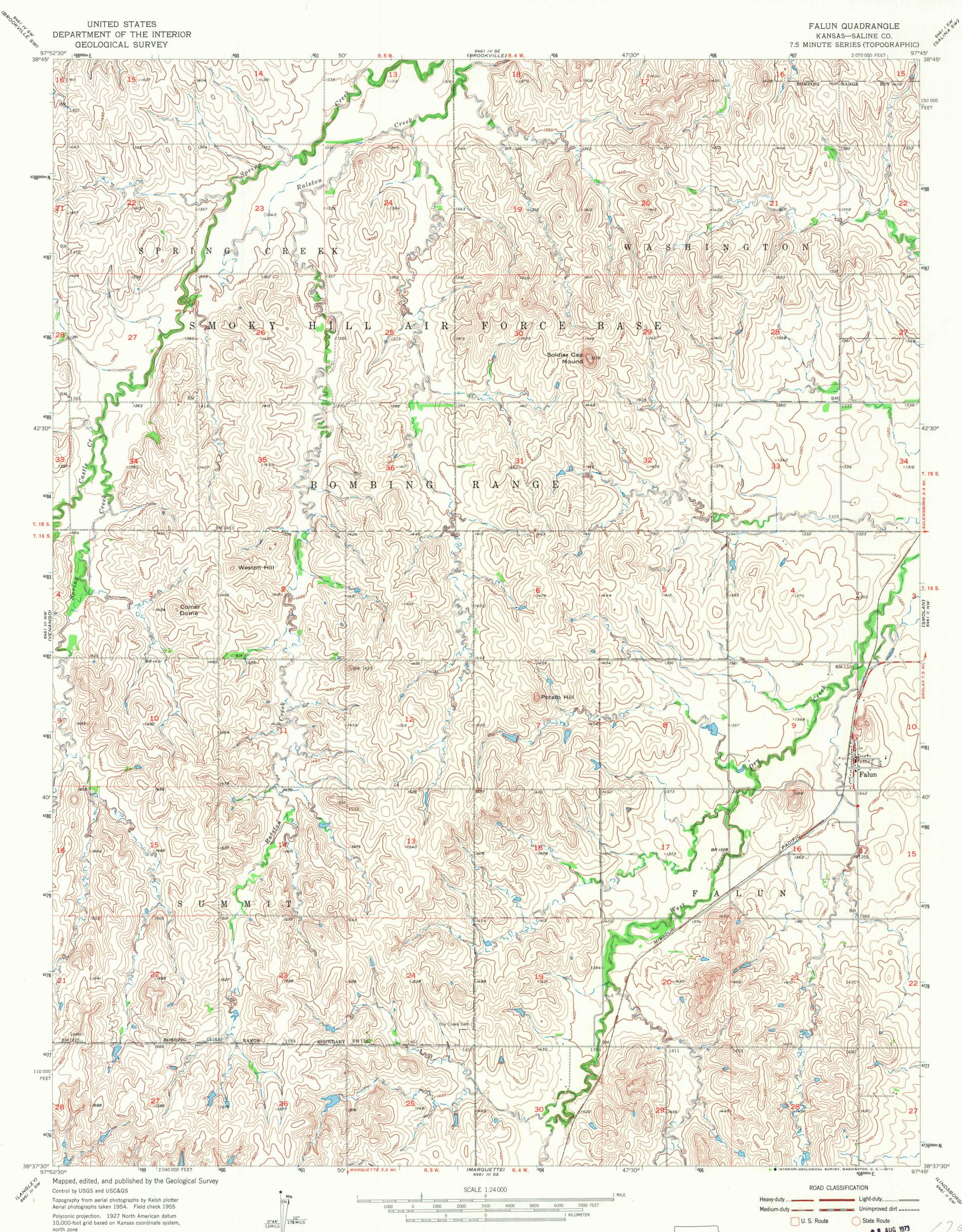
Polyconic projection. 1927 North American datum 10,000-foot grid based on Kansas coordinate system, north zone 1000-meter Universal Transverse Mercator grid ticks, zone 14, shown in blue
