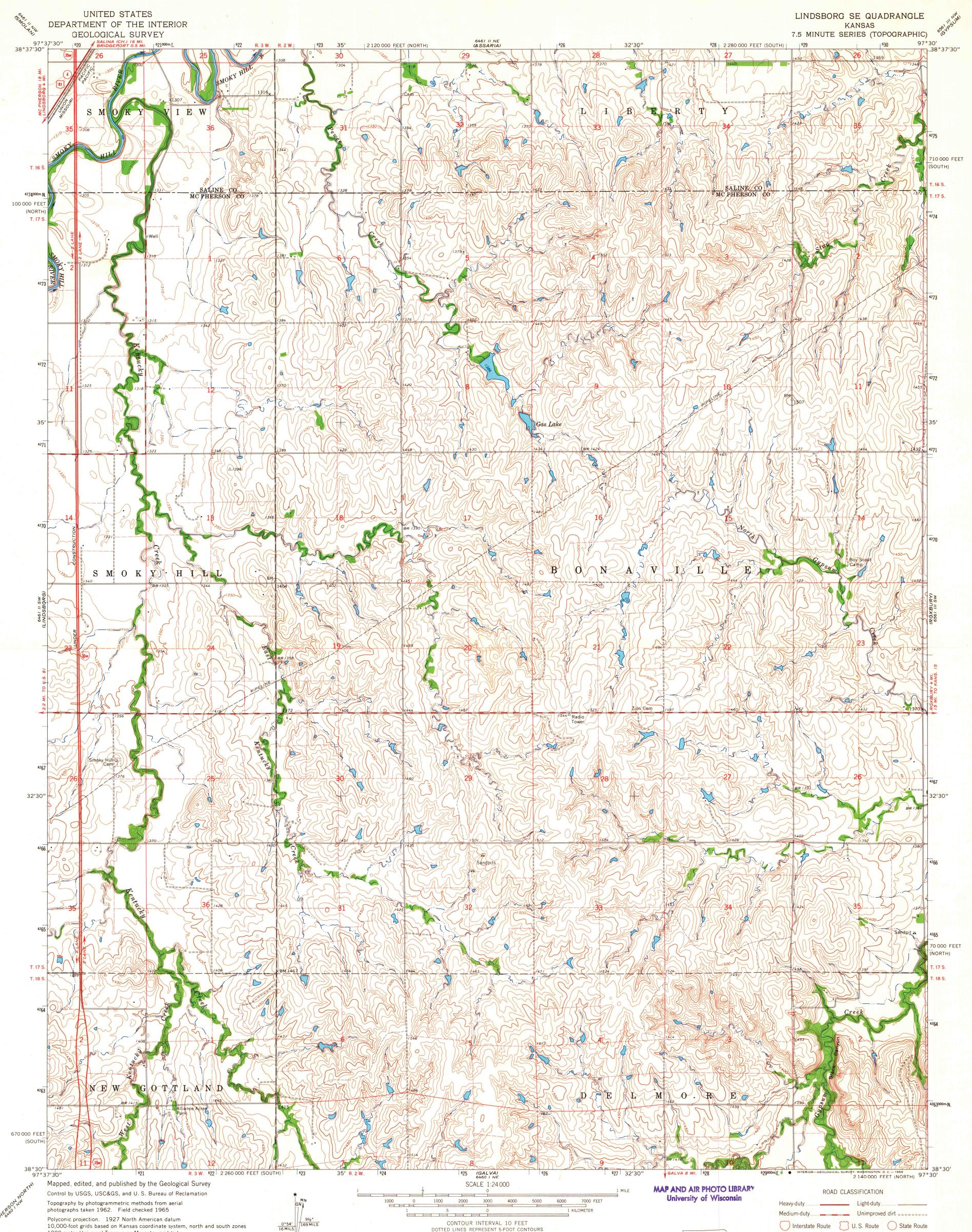
Polyconic projection. 1927 North American datum 10,000-foot grids based on Kansas coordinate system, north and south zones 1000-meter Universal Transverse Mercator grid ticks, zone 14, shown in blue
