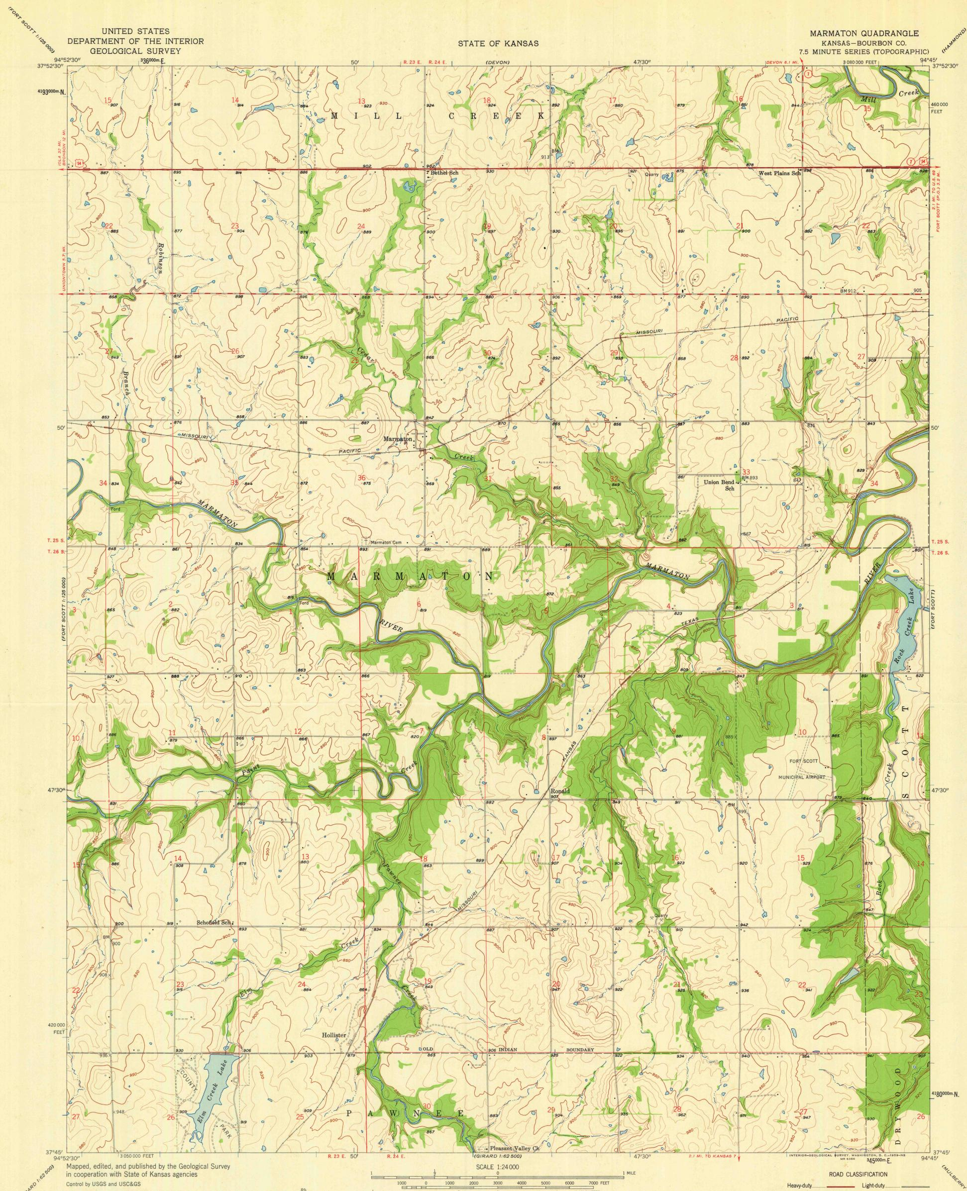
Control by USGS and USC&GS Topography from aerial photographs by Kelsh plotter Aerial photographs taken 1957. Field check 1958 Polyconic projection. 1927 North American datum 10,000-foot grid based on Kansas coordinate system, south zone 1000-meter Universal Transverse Mercator grid ticks, zone 15, shown in blue
