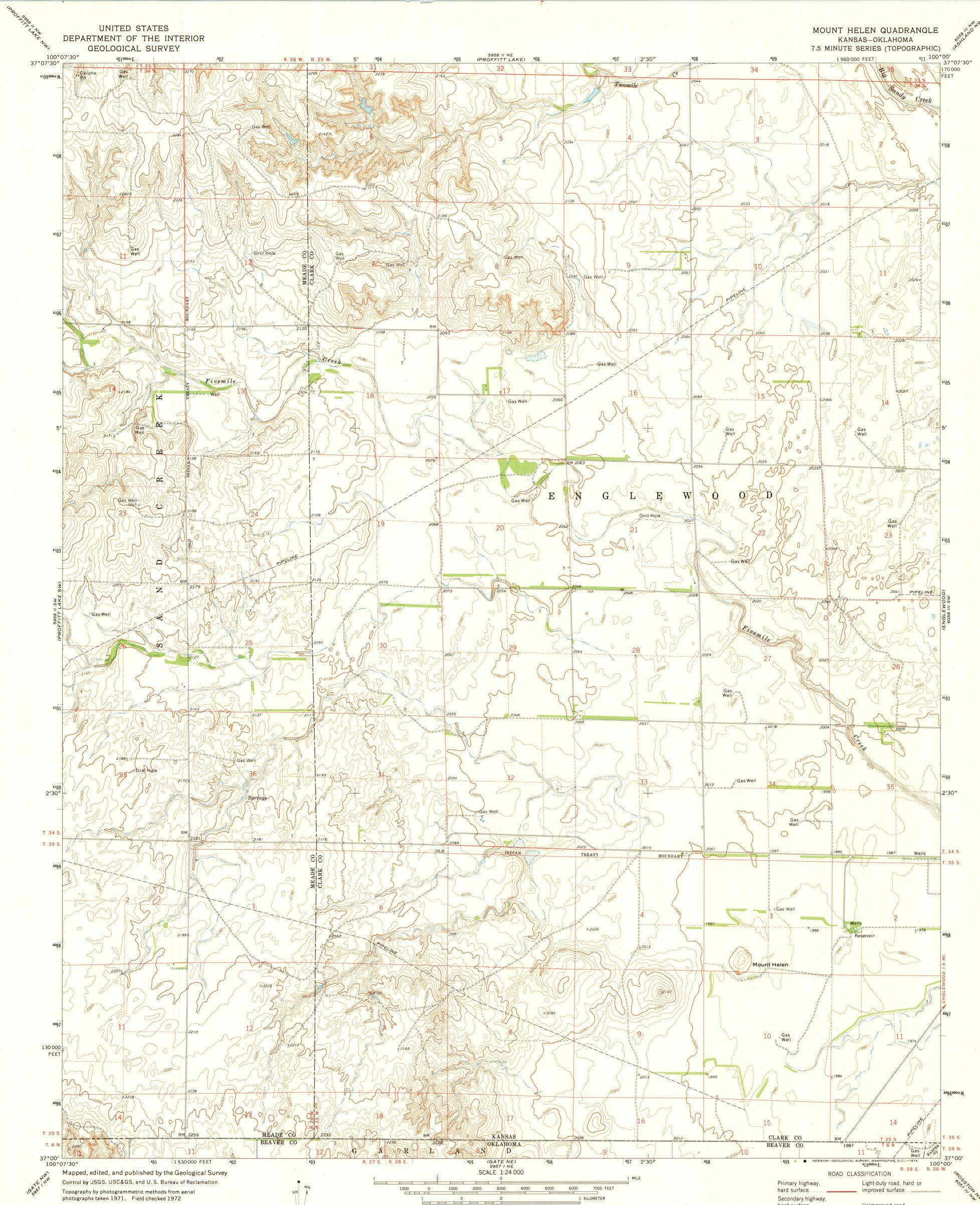
Projection and 10,000-foot grid ticks: Kansas coordinate system, south zone (Lambert conformal conic) 1000-meter Universal Transverse Mercator grid ticks, zone 14, shown in blue. 1927 North American datum
