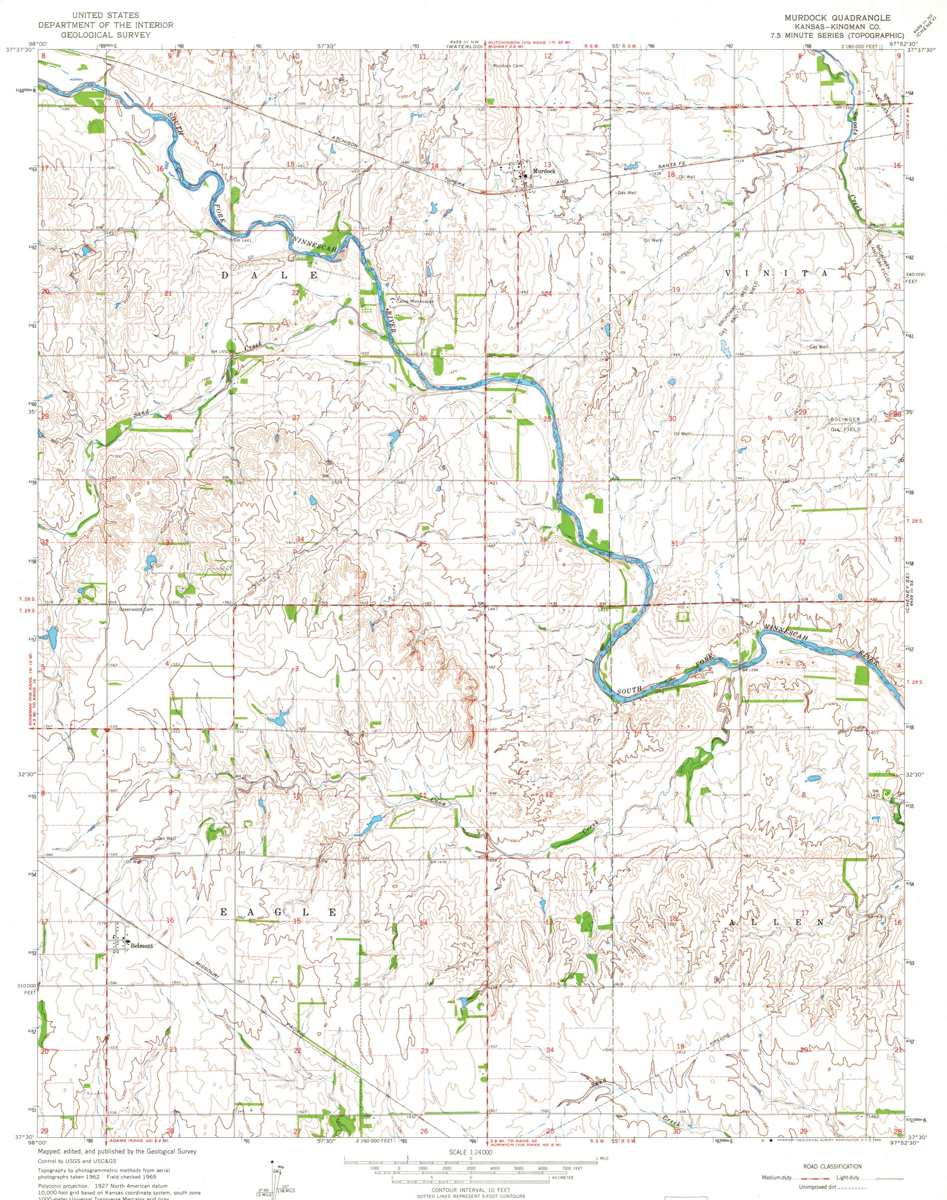
Polyconic projection. 1927 North American datum 10,000-foot grid based on Kansas coordinate system, south zone 1000-meter Universal Transverse Mercator grid ticks, zone 14, shown in blue
