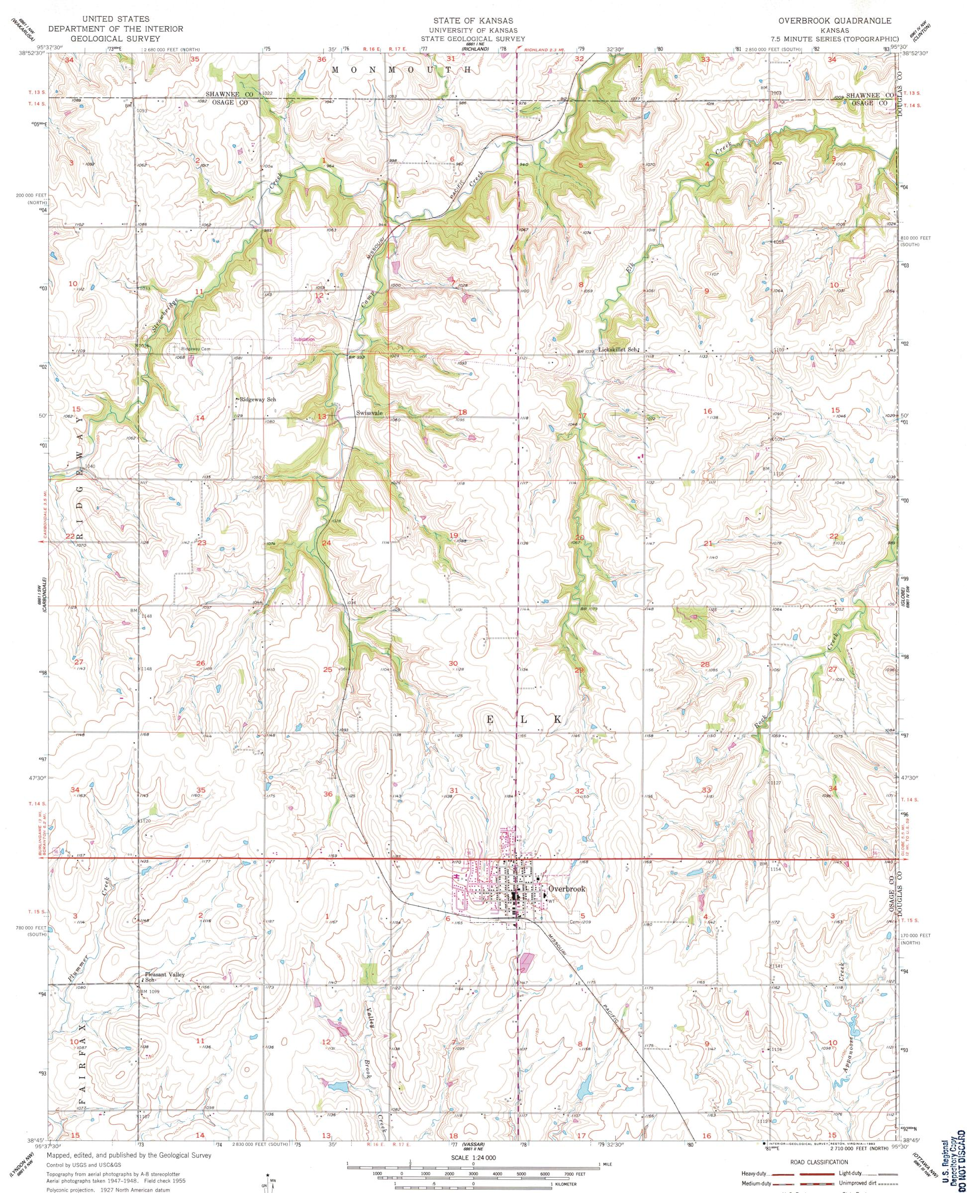
Polyconic projection. 1927 North American datum 10,000-foot grids based on Kansas coordinate system, north and south zones 1000-meter Universal Transverse Mercator grid ticks, zone 15, shown in blue To place on the predicted North American Datum 1983, move the projection lines 2 meters north and 23 meters east as shown by dashed corner ticks
