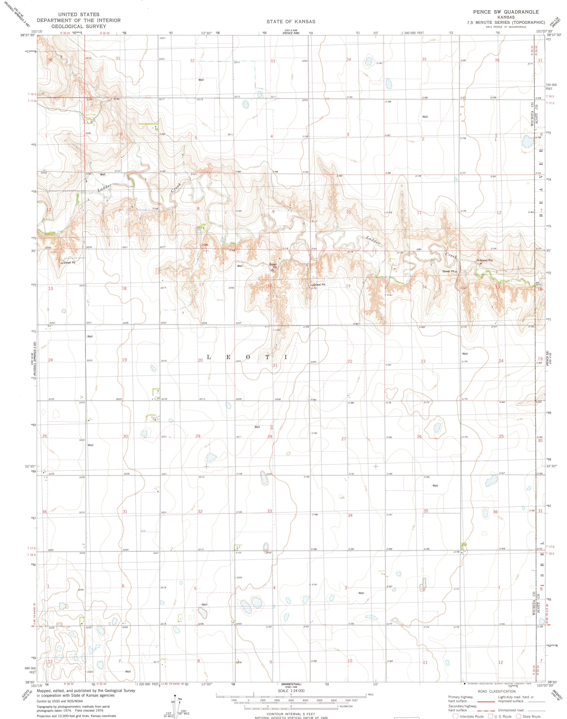
Projection and 10,000-foot grid ticks: Kansas coordinate system, south zone (Lambert conformal conic) 1000-meter Universal Transverse Mercator grid, zone 14 1927 North American datum
