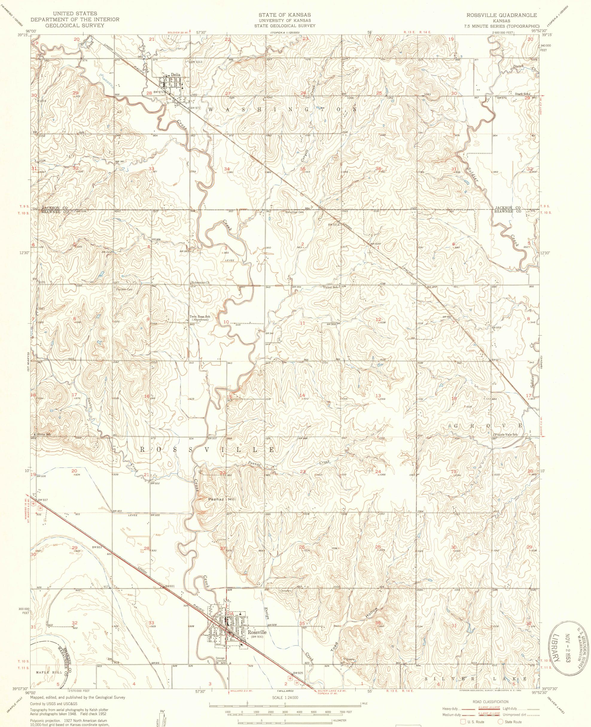
Polyconic projection. 1927 North American datum 10,000-foot grid based on Kansas coordinate system, north zone
