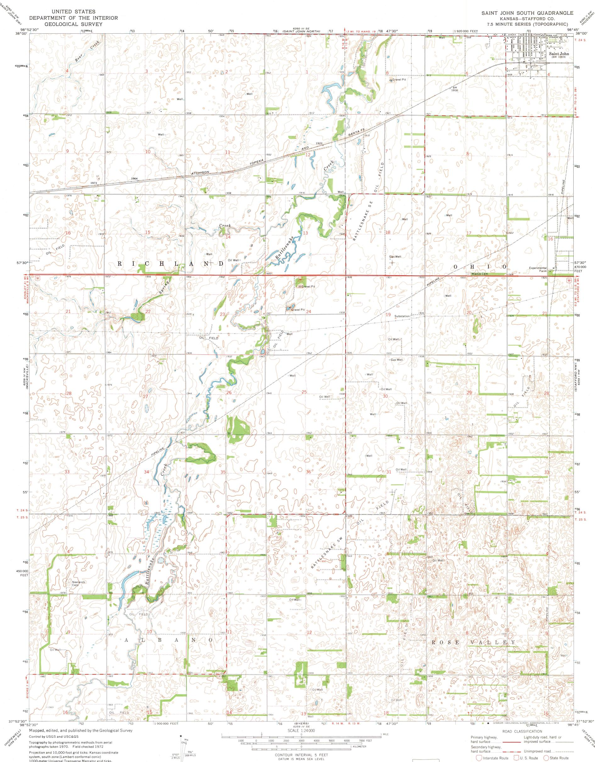
Projection and 10,000-foot grid ticks: Kansas coordinate system, south zone (Lambert conformal conic) 1000-meter Universal Transverse Mercator grid ticks, zone 14, shown in blue. 1927 North American datum
