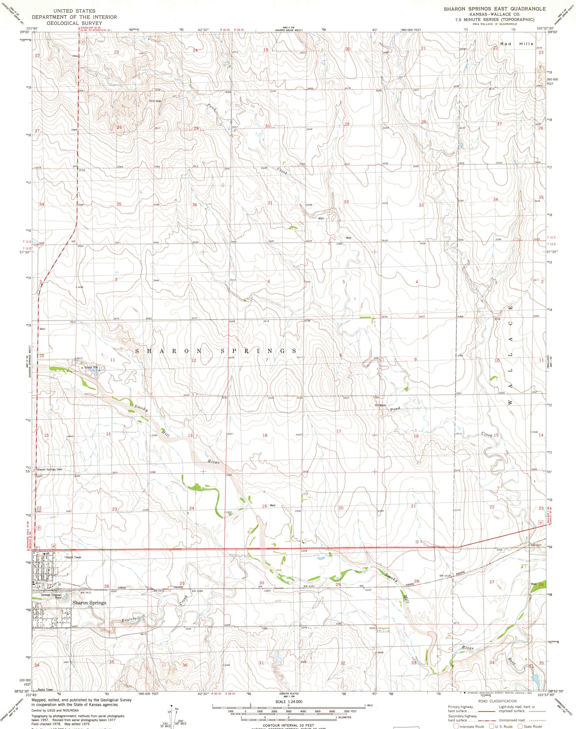
Projection and 10,000-foot grid ticks: Kansas coordinate system, north zone (Lambert conformal conic) 1000-meter Universal Transverse Mercator grid, zone 14 1927 North American datum To place on the predicted North American Datum 1983 move the projection lines 3 meters north and 39 meters east as shown by dashed corner ticks
