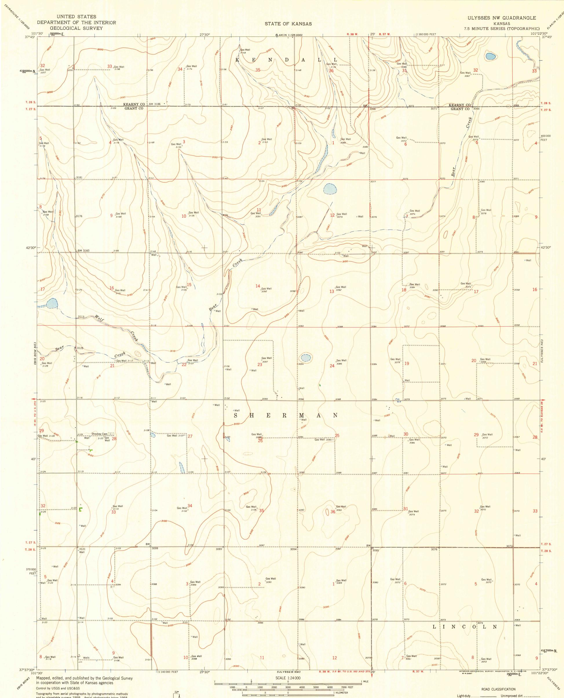
and by planetable surveys 1959. Aerial photographs taken 1958 Polyconic projection. 1927 North American datum 10,000-foot grid based on Kansas coordinate system, south zone 1000-meter Universal Transverse Mercator grid ticks, zone 14, shown in blue
