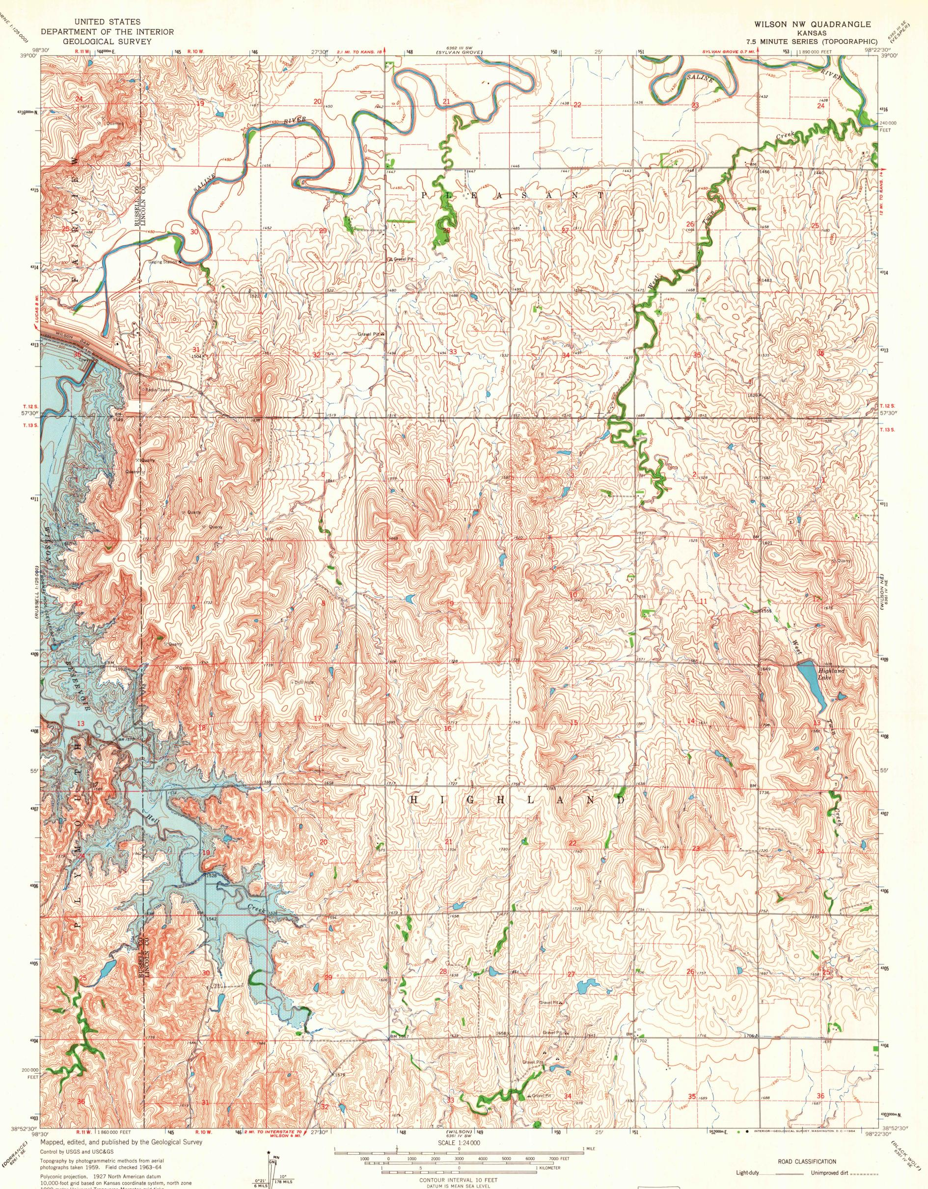
10,000-foot grid based on Kansas coordinate system, north zone 1000-meter Universal Transverse Mercator grid ticks, zone 14, shown in blue
