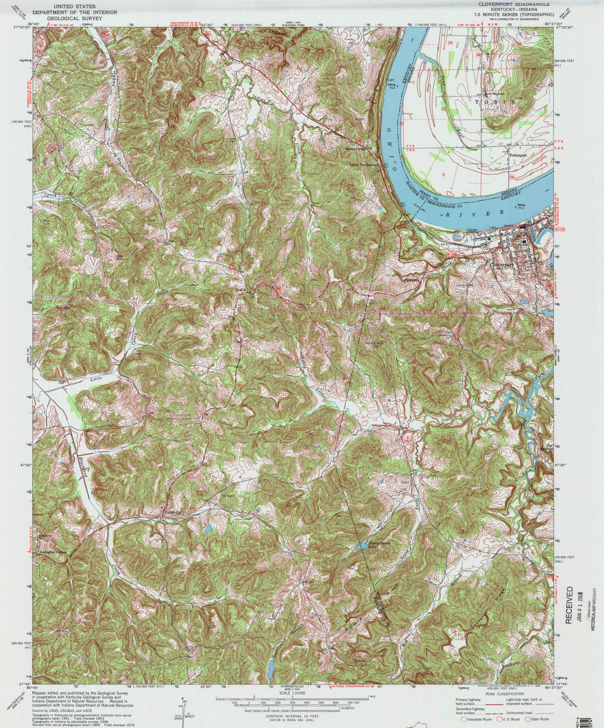
Polyconic projection. 1927 North American datum 10,000-foot grids based on Kentucky coordinate system, south zone, and Indiana coordinate system, west zone 1000-meter Universal Transverse Mercator grid ticks, zone 16, shown in blue
