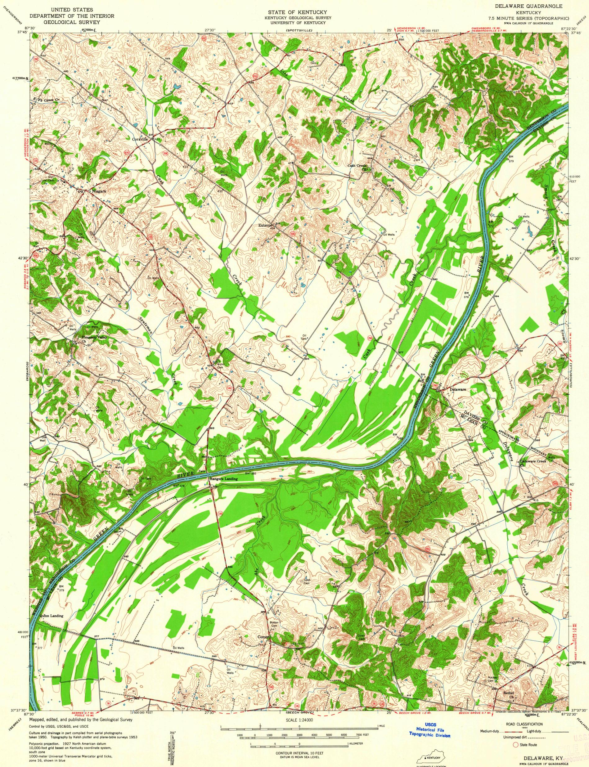
Polyconic projection. 1927 North American datum 10,000-foot grid based on Kentucky coordinate system, south zone 1000-meter Universal Transverse Mercator grid ticks, zone 16, shown in blue
