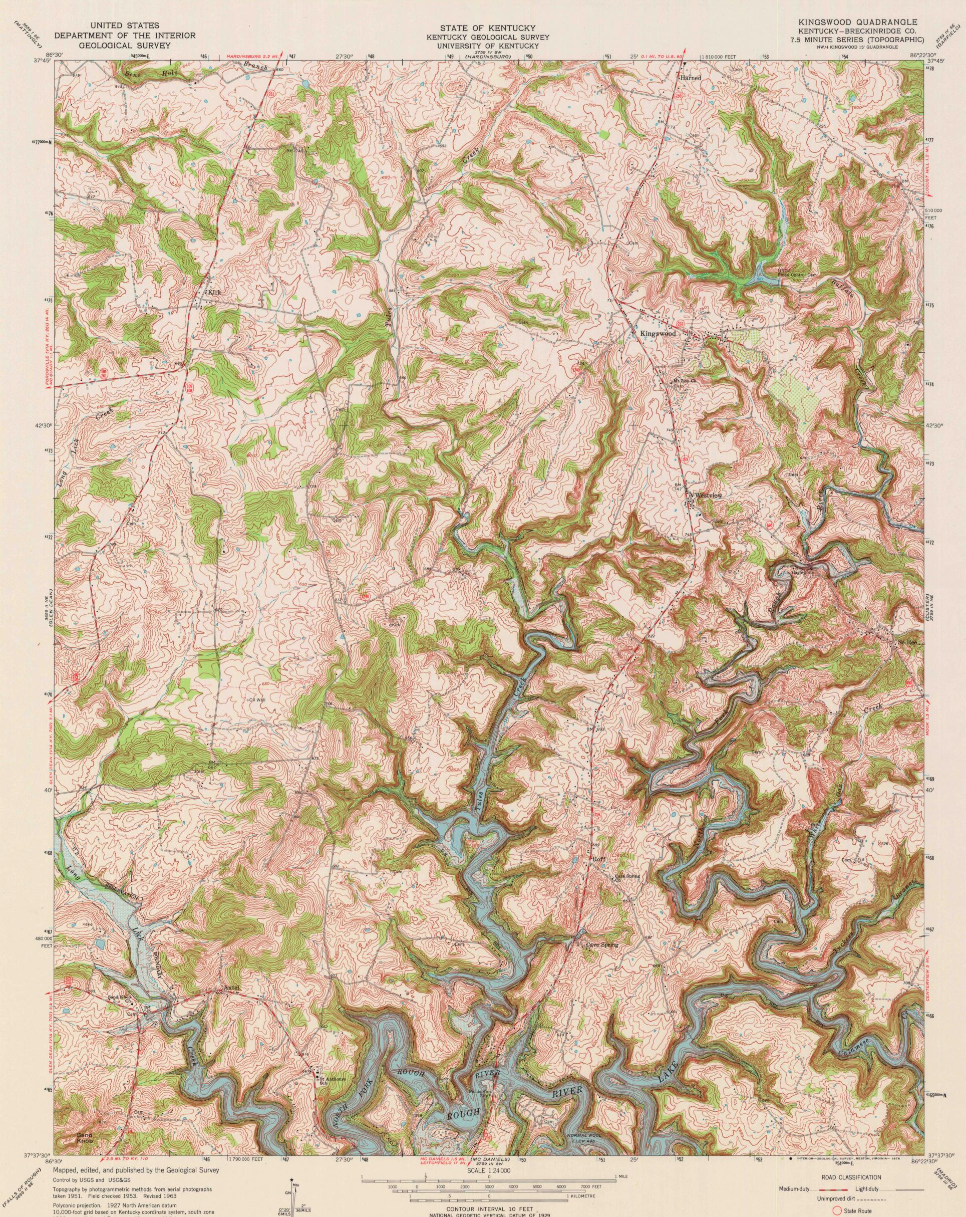
Polyconic projection. 1927 North American datum 10,000-foot grid based on Kentucky coordinate system, south zone 1000-metre Universal Transverse Mercator grid ticks, zone 16, shown in blue
