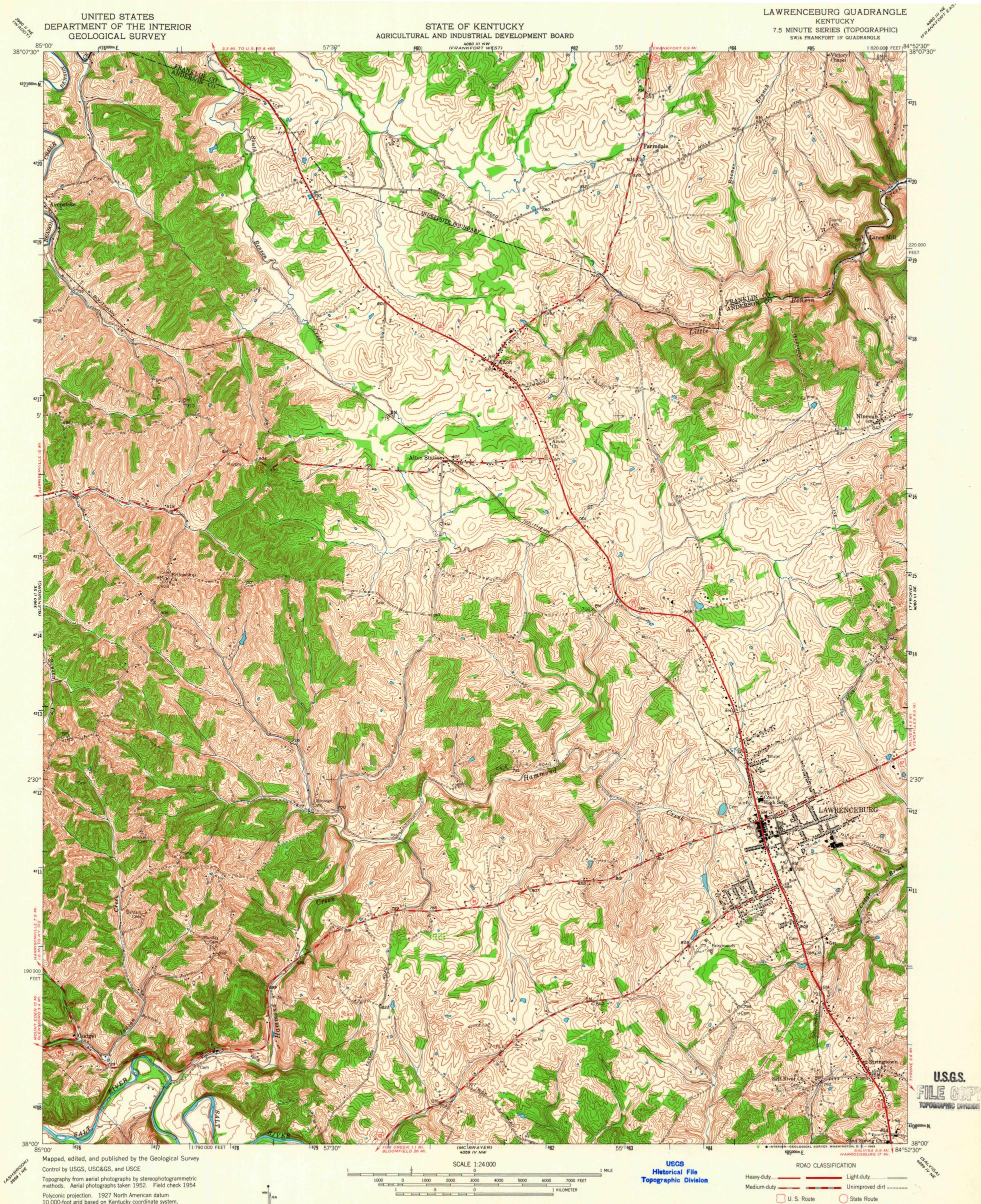
10,000-foot grid based on Kentucky coordinate system, north zone
