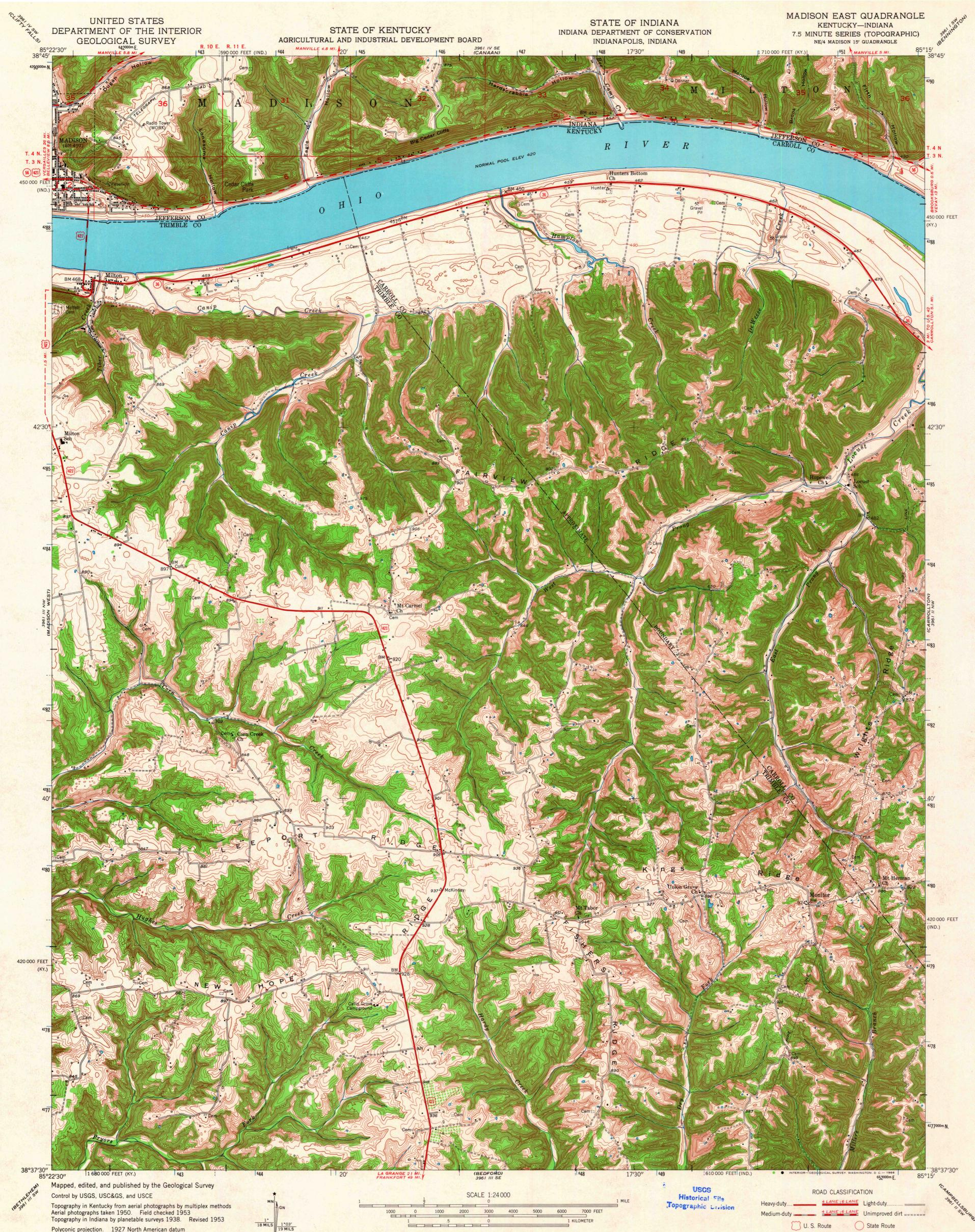
Polyconic projection. 1927 North American datum 10,000-foot grids based on Kentucky coordinate system, north zone, and Indiana coordinate system, east zone 1000-meter Universal Transverse Mercator grid ticks, zone 16, shown in blue
