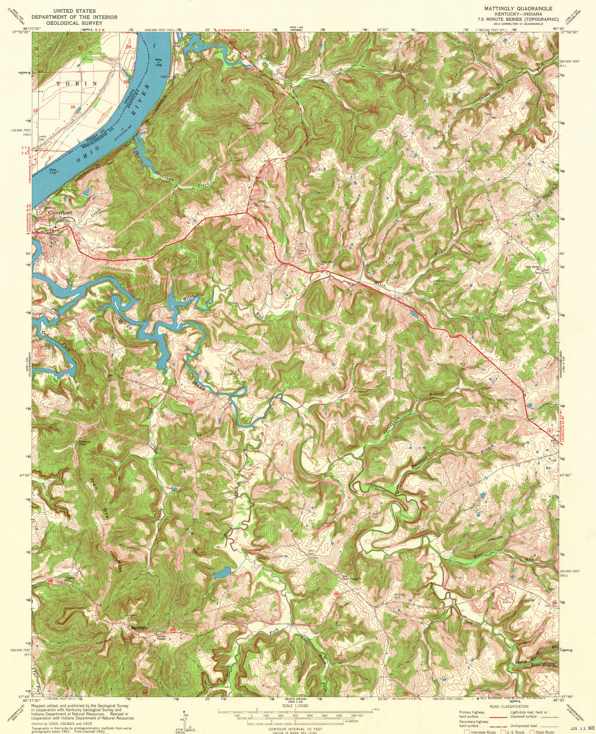
Topography in Kentucky by photogrammetric methods from aerial photographs taken 1951. Field checked 1953 Topography in Indiana by planetable surveys 1946 Revised from aerial photographs taken 1969. Field checked 1970
