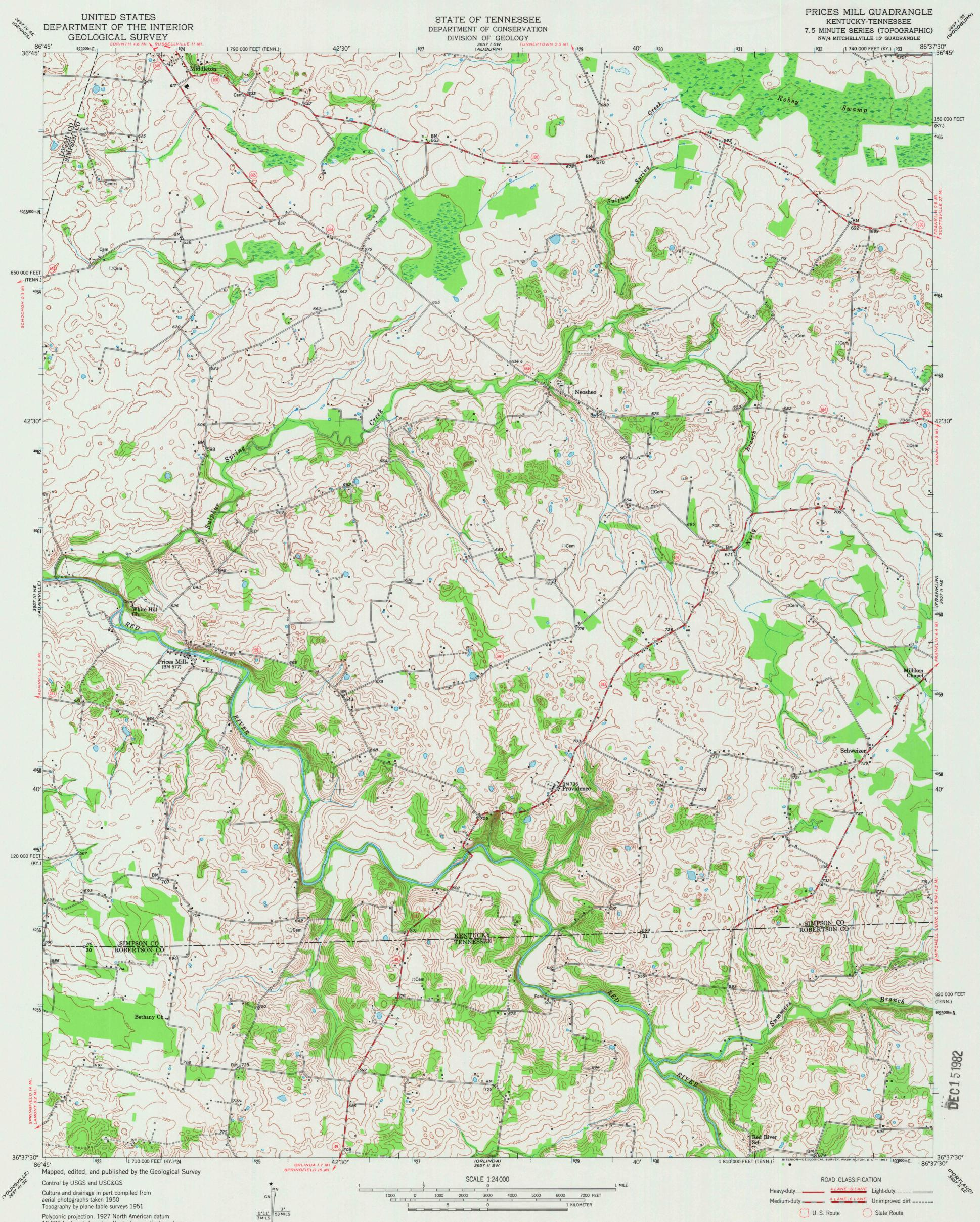
Polyconic projection. 1927 North American datum 10,000-foot grids based on Kentucky coordinate system, south zone, and Tennessee coordinate system 1000-meter Universal Transverse Mercator grid ticks, zone 16, shown in blue
