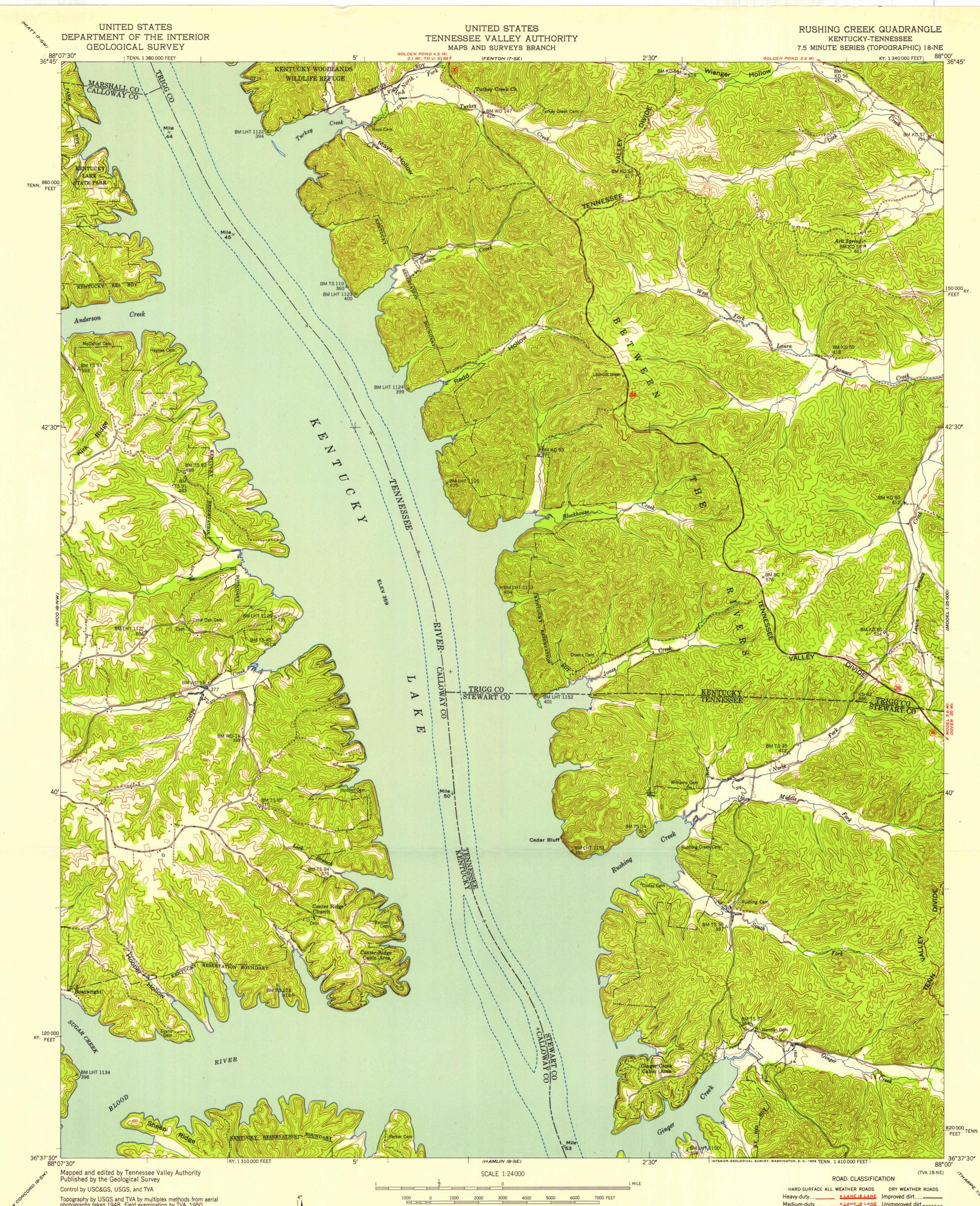
Topography by USGS and TVA by multiplex methods from aerial photographs taken 1948. Field examination by TVA, 1950
