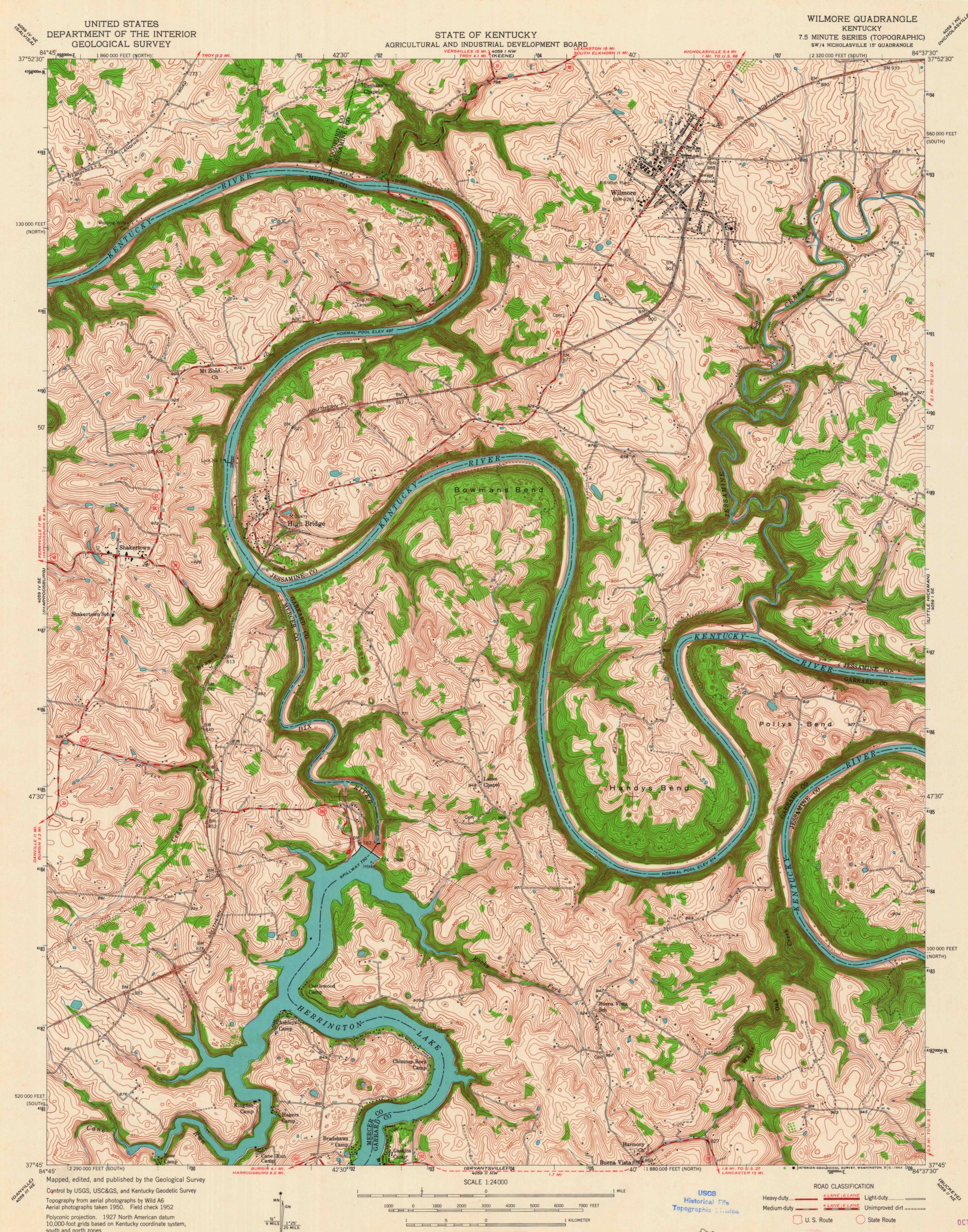
Polyconic projection. 1927 North American datum 10,000-foot grids based on Kentucky coordinate system, south and north zones 1000-meter Universal Transverse Mercator grid ticks, zone 16, shown in blue
