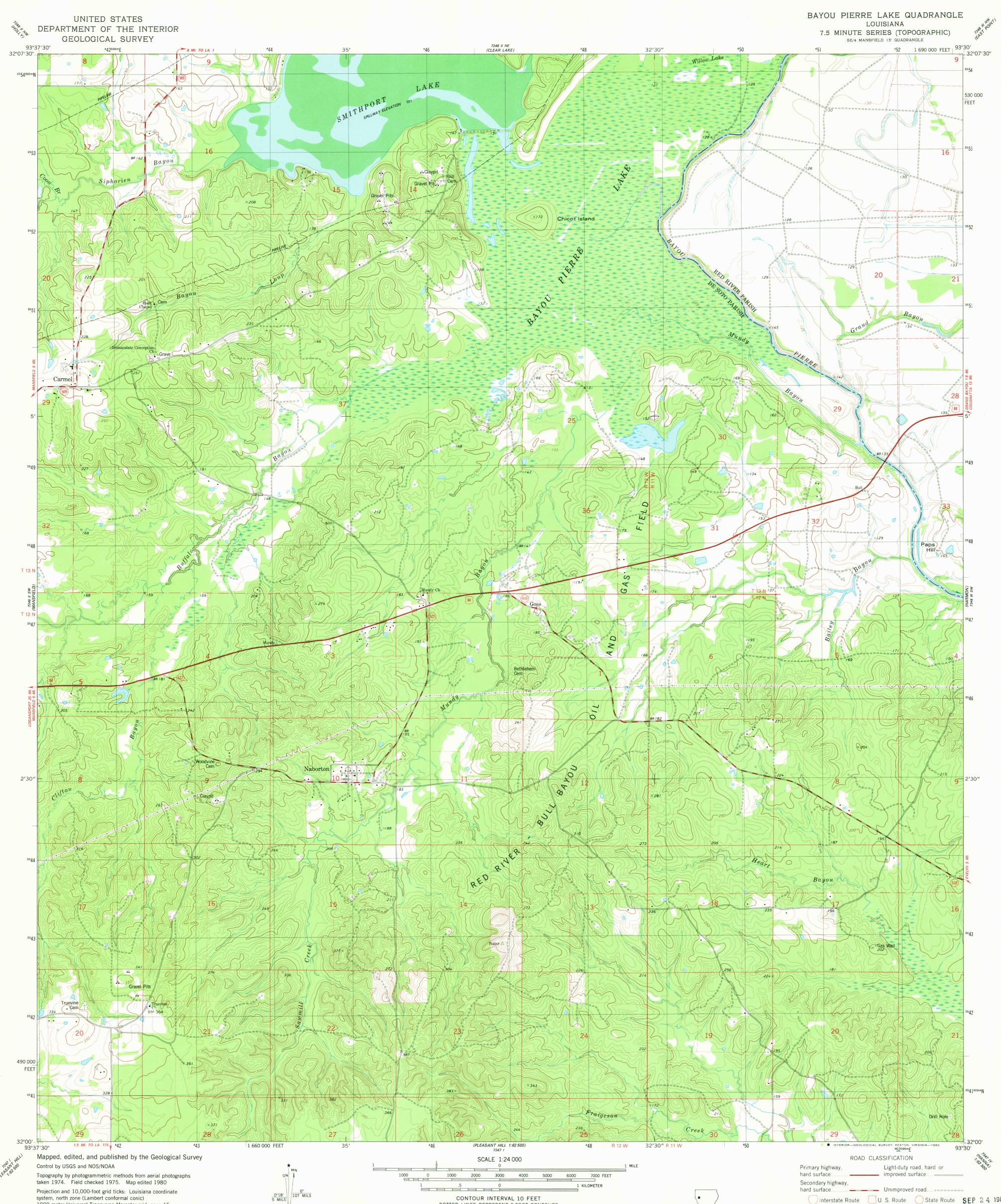
Projection and 10,000-foot grid ticks: Louisiana coordinate system, north zone (Lambert conformal conic) 1000-meter Universal Transverse Mercator grid, zone 15 1927 North American Datum To place on the predicted North American Datum 1983 move the projection lines 14 meters south and 17 meters east as shown by dashed corner ticks
