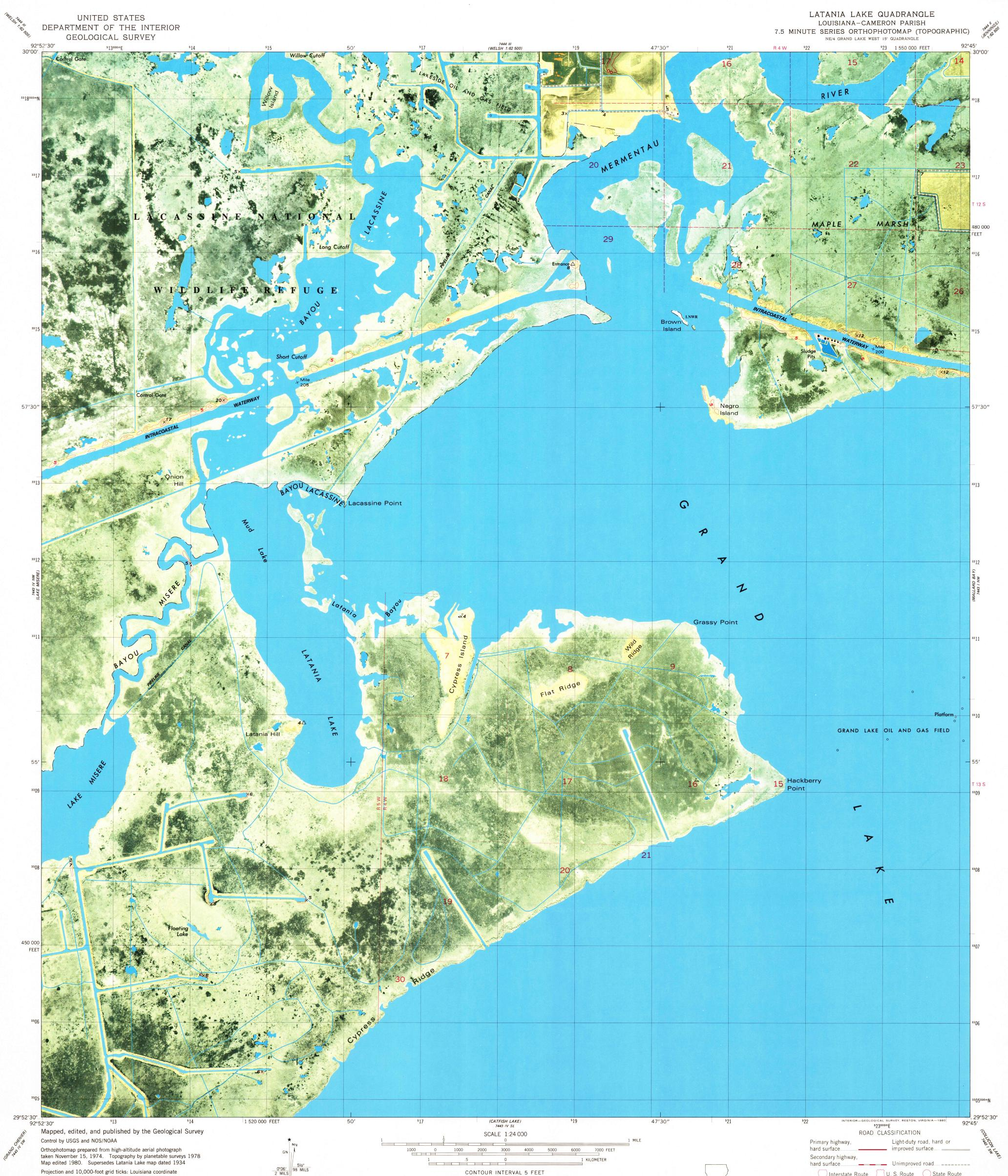
system, south zone (Lambert conformal conic) 1000-meter Universal Transverse Mercator grid, zone 15 1927 North American Datum To place on the predicted North American Datum 1983 move the projection lines 19 meters south and 15 meters east as shown by dashed corner ticks All or part of this quadrangle lies within a subsidence area There may be private inholdings within the boundaries of the National or State reservations shown on this map
