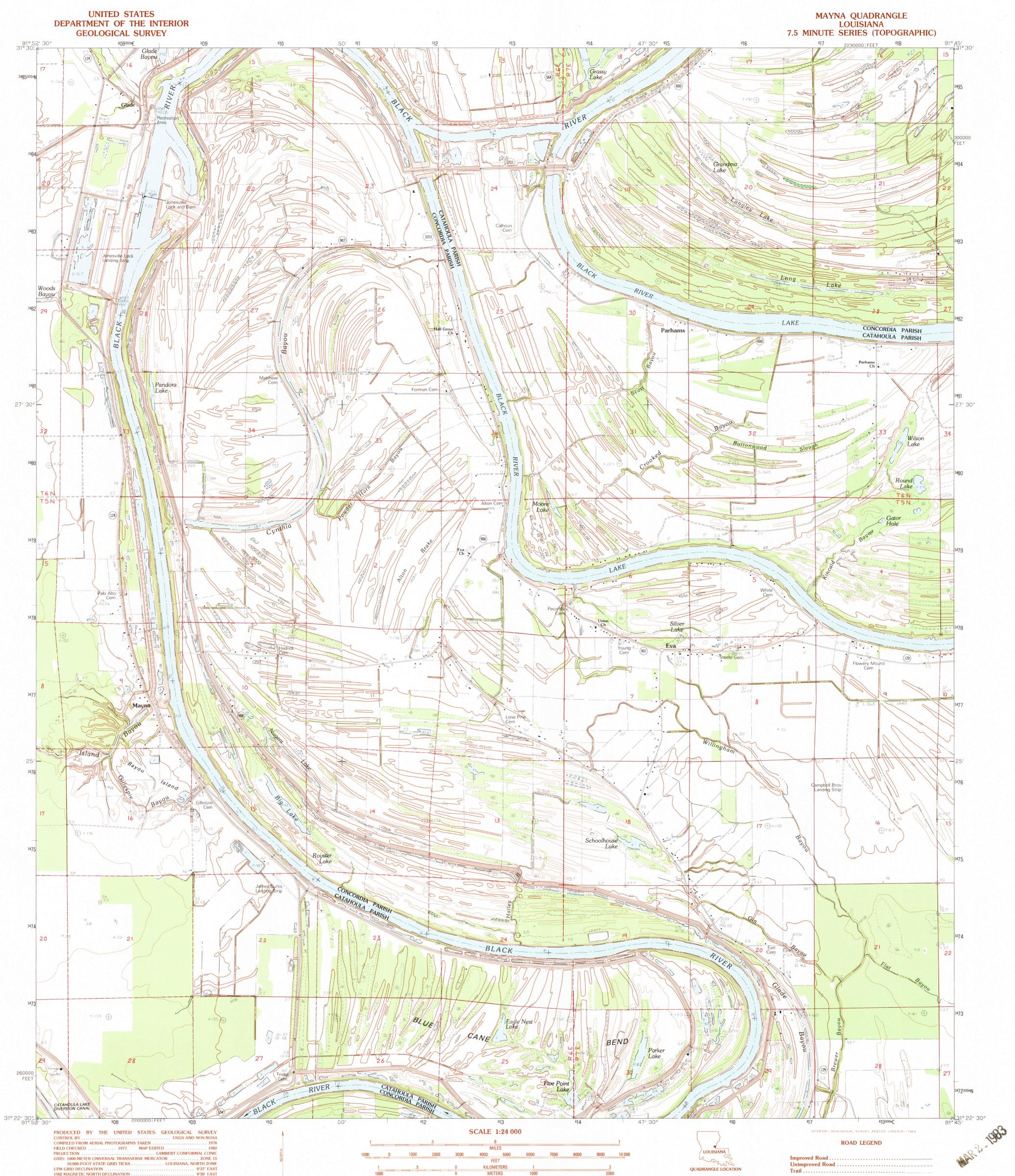
1982 MAGNETIC NORTH DECLINATION ... VERTICAL DATUM ...... NATIONAL GEODETIC VERTICAL DATUM OF 1929 ..... 1927 NORTH AMERICAN DATUM HORIZONTAL DATUM ..... To place on the predicted North American Datum of 1983 move the projection lines as shown by dashed corner ticks (15 meters south and 12 meters east)
