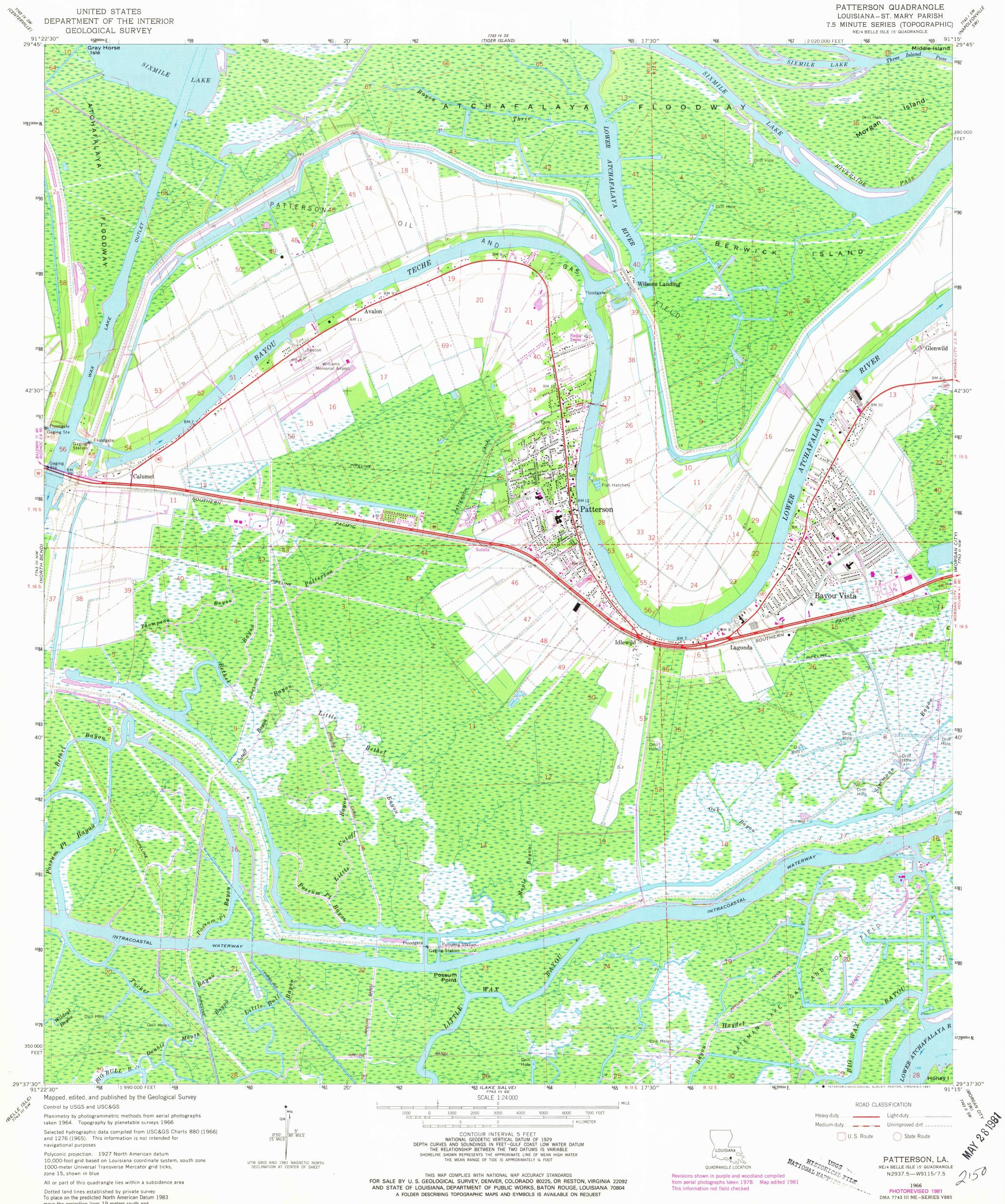
move the projection lines 19 meters south and 11 meters east as shown by dashed corner ticks
