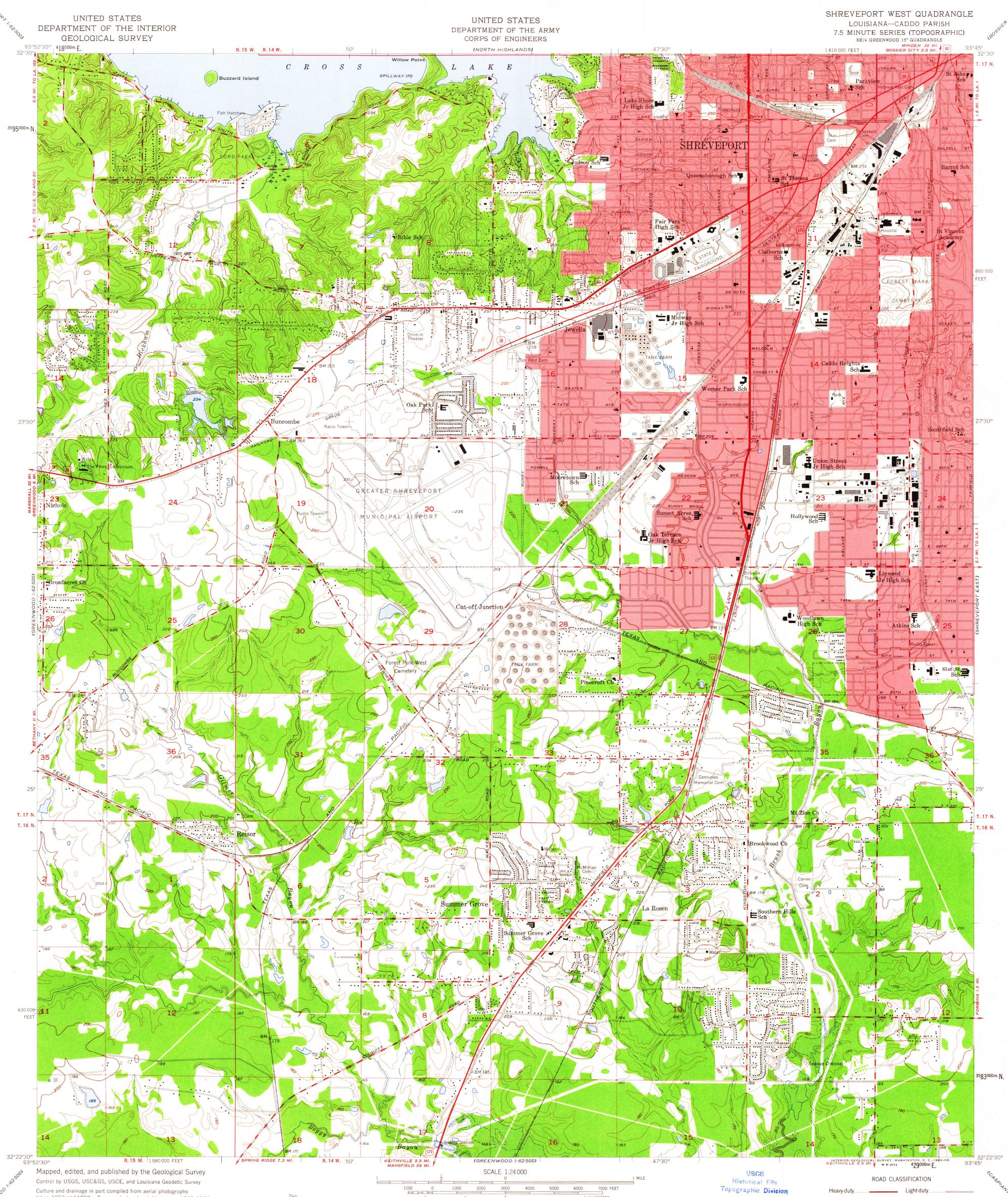
taken 1952 and 1959. Topography by planetable surveys 1942–1943 and 1955. Revised 1959 Polyconic projection. 1927 North American datum 10,000-foot grid based on Louisiana coordinate system, north zone 1000-meter Universal Transverse Mercator grid ticks, zone 15, shown in blue Red tint indicates areas in which only landmark buildings are shown Broken light-blue lines indicate area subject to inundation above Wallace Lake Dam
