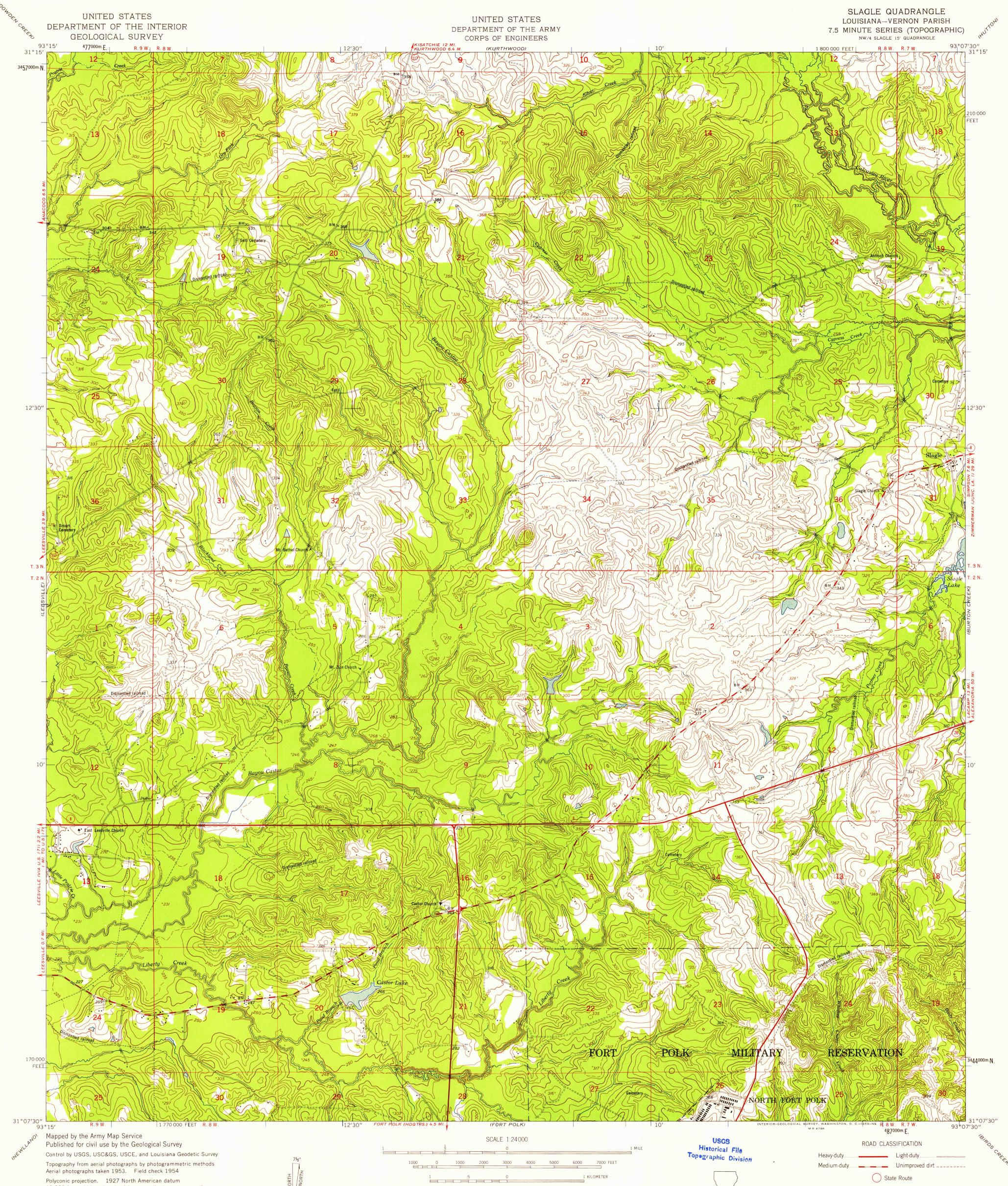
Polyconic projection. 1927 North American datum 10,000-foot grid based on Louisiana coordinate system, north zone 1000-meter Universal Transverse Mercator grid ticks, zone 15, shown in blue Unchecked elevations are shown in brown
