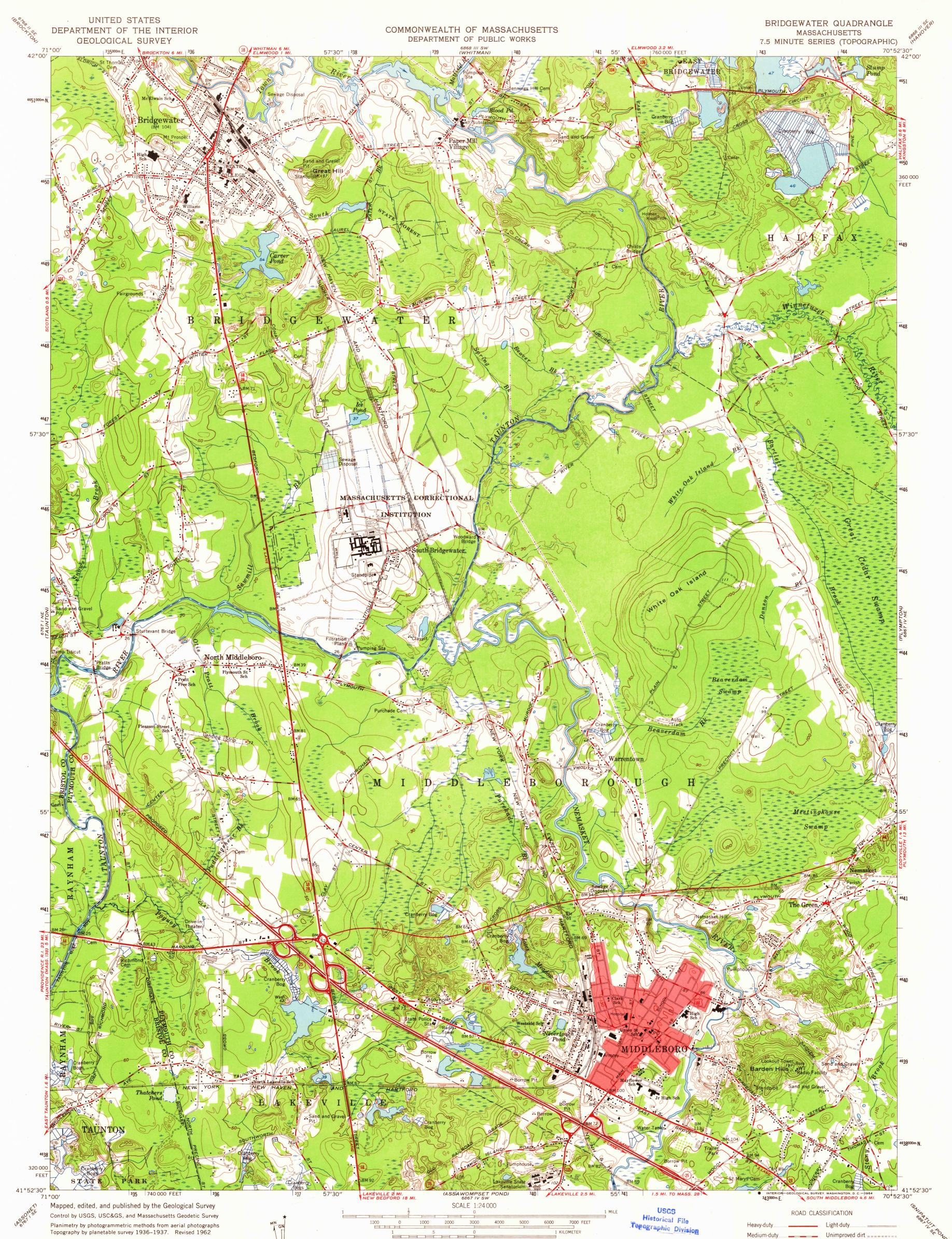
Polyconic projection. 1927 North American datum 10,000-foot grid based on Massachusetts coordinate system, mainland zone 1000-meter Universal Transverse Mercator grid ticks, zone 19, shown in blue
