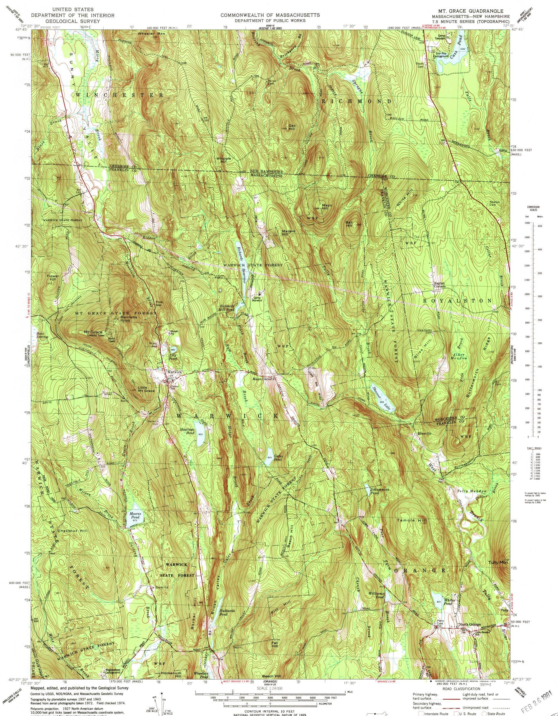
10,000-foot grid ticks based on Massachusetts coordinate system, mainland zone, and New Hampshire coordinate system 1000-meter Universal Transverse Mercator grid, zone 18
