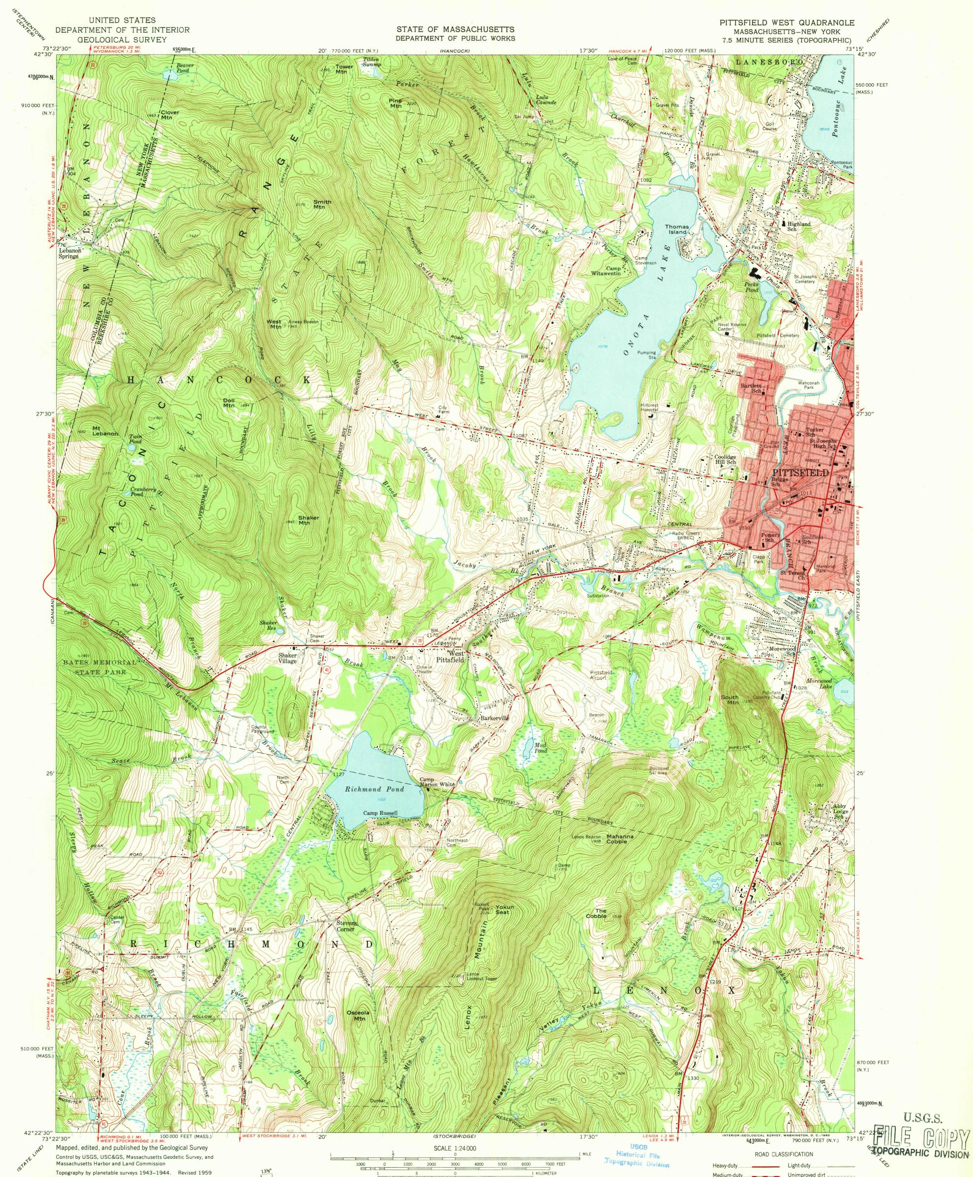
Polyconic projection. 1927 North American datum 10,000-foot grids based on Massachusetts coordinate system, mainland zone, and New York coordinate system, east zone 1000-meter Universal Transverse Mercator grid ticks, zone 18, shown in blue Fine red dashed lines indicate selected fence and field lines visible on aerial photographs. This information is unchecked
