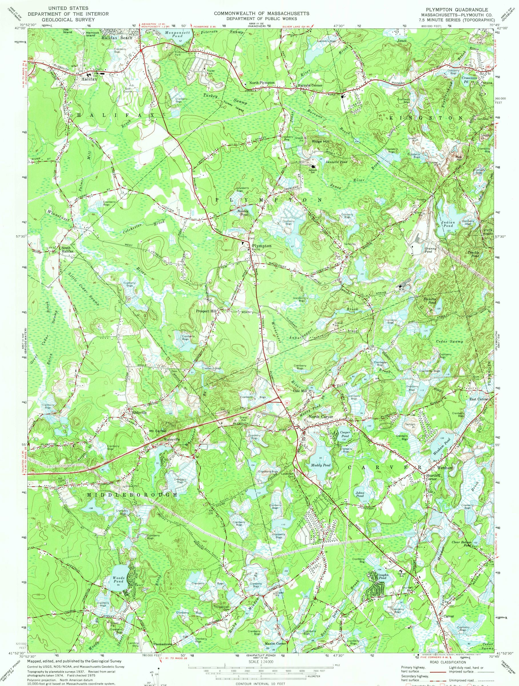
10,000-foot grid based on Massachusetts coordinate system, mainland zone 1000-metre Universal Transverse Mercator grid ticks, zone 19, shown in blue
