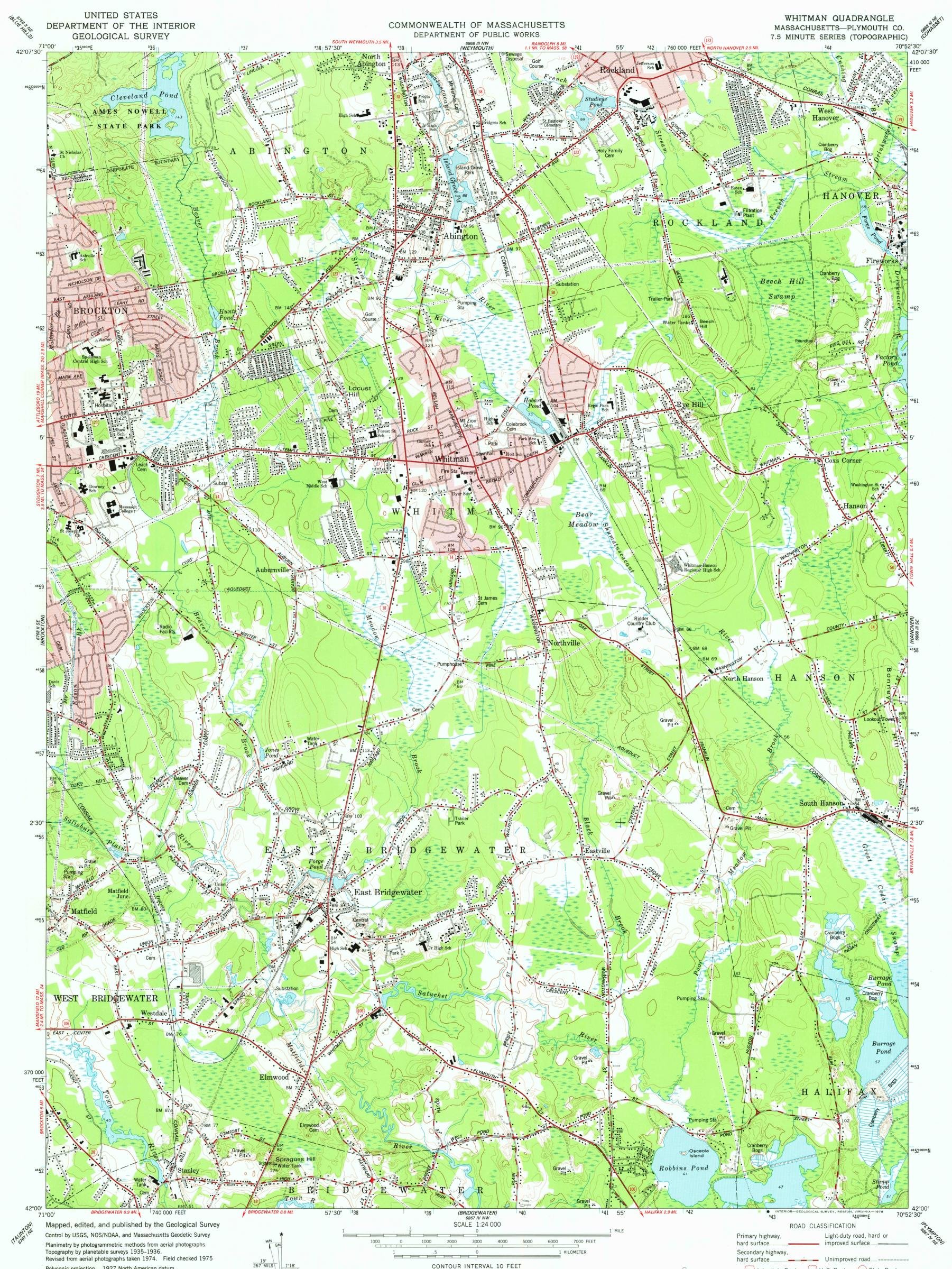
Polyconic projection. 1927 North American datum 10,000-foot grid ticks based on Massachusetts coordinate system, mainland zone 1000-meter Universal Transverse Mercator grid ticks, zone 19, shown in blue Red tint indicates areas in which only landmark buildings are shown
