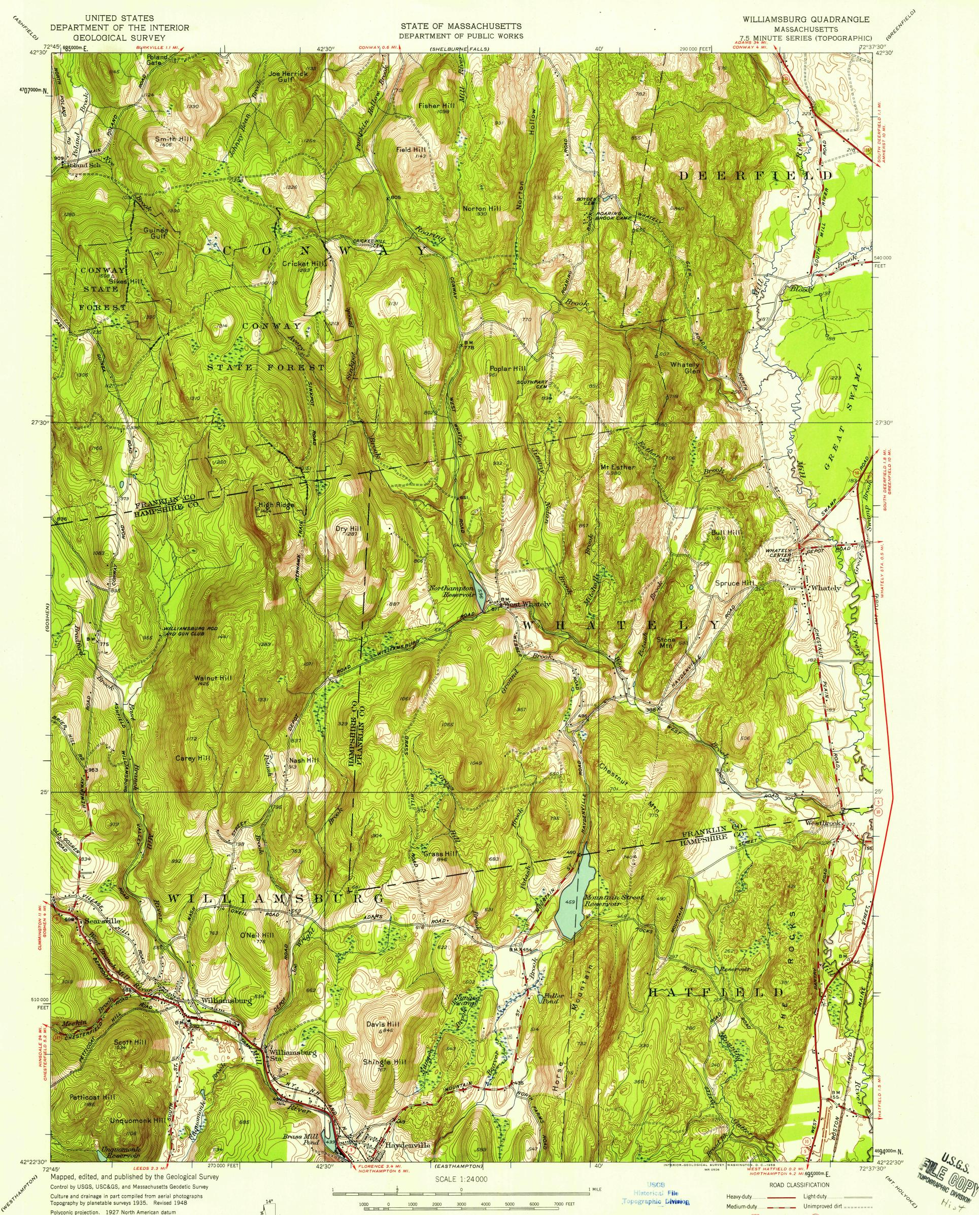
10,000-foot grid based on Massachusetts (Mainland) coordinate system 1000-meter Universal Transverse Mercator grid ticks, zone 18, shown in blue
