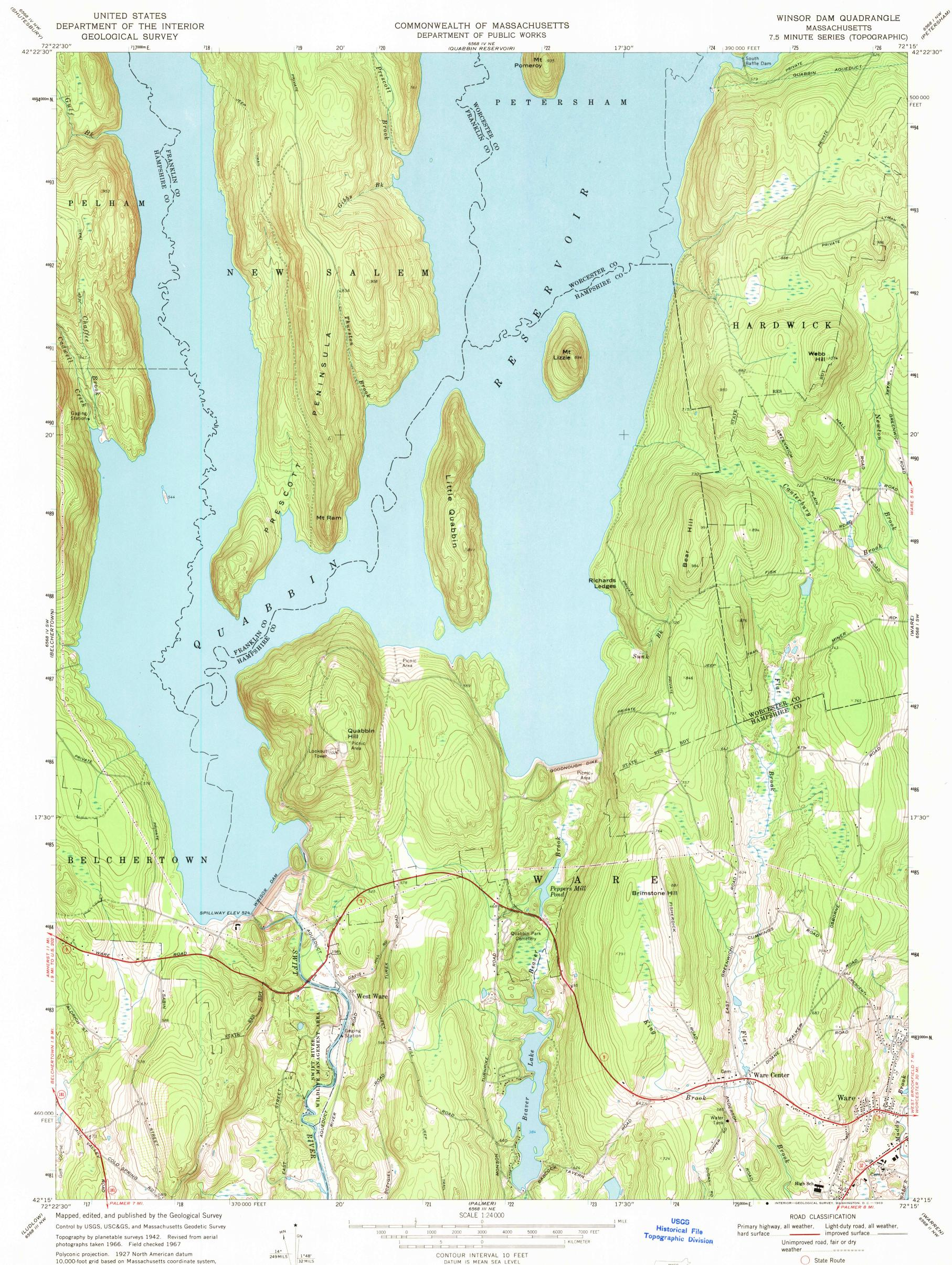
249 MILS 10,000-foot grid based on Massachusetts coordinate system, mainland zone 1000-meter Universal Transverse Mercator grid ticks, zone 18, shown in blue UTM GRID AND 1967 MAGNETIC NORTH DECLINATION AT CENTER OF SHEET Fine red dashed lines indicate selected fence and field lines where generally visible on aerial photographs. This information is unchecked
