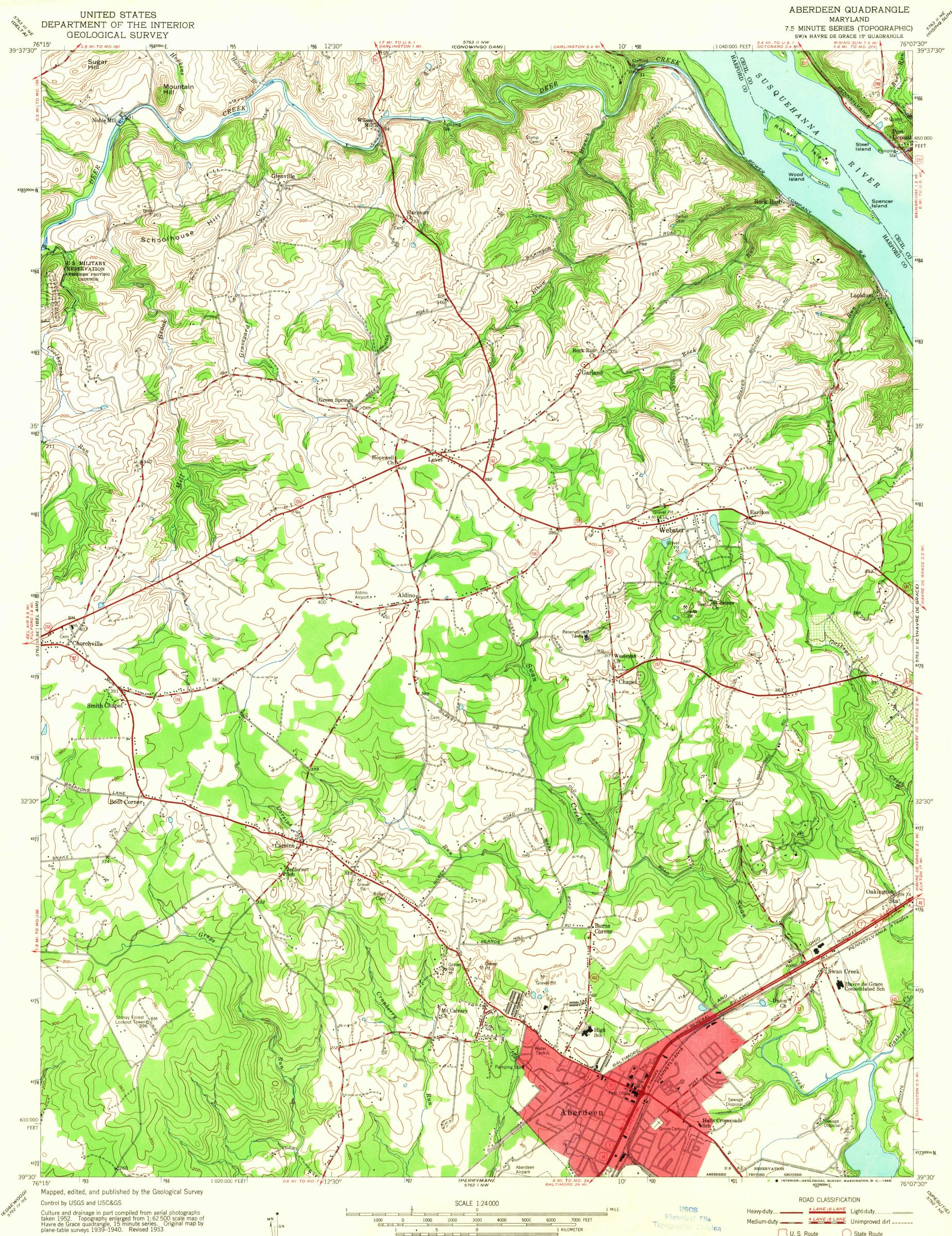
Polyconic projection. 1927 North American datum 10,000-foot grid based on Maryland coordinate system 8° 142 MILS 0°45' 13 MILS Red tint indicates area in which only Iandmark buildings are shown 1000-meter Universal Transverse Mercator grid ticks, UTM GRID AND 1953 MAGNETIC NORTH DECLINATION AT CENTER OF SHEET zone 18, shown in blue
