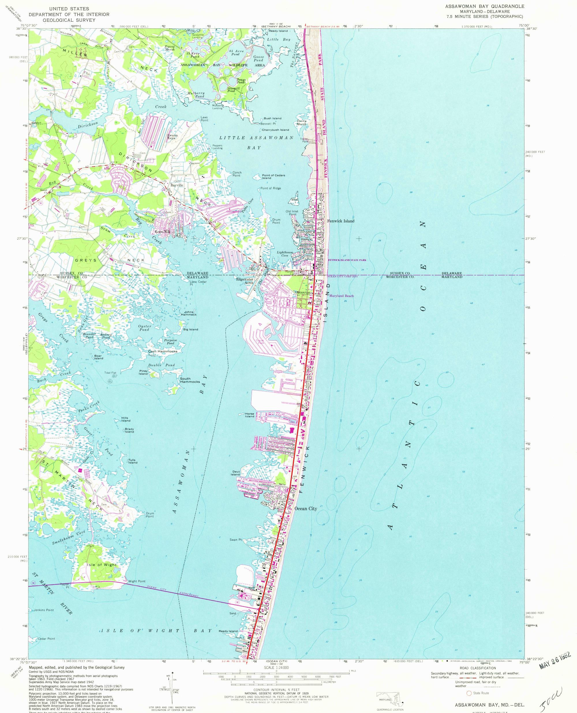
Polyconic projection. 10,000-foot grid ticks based on Maryland coordinate system, and Delaware coordinate system. 1000-meter Universal Transverse Mercator grid ticks, zone 18, shown in blue. 1927 North American Datum. To place on the predicted North American Datum 1983 move the projection lines 8 meters south and 32 meters west as shown by dashed corner ticks These methods are the standard standa
