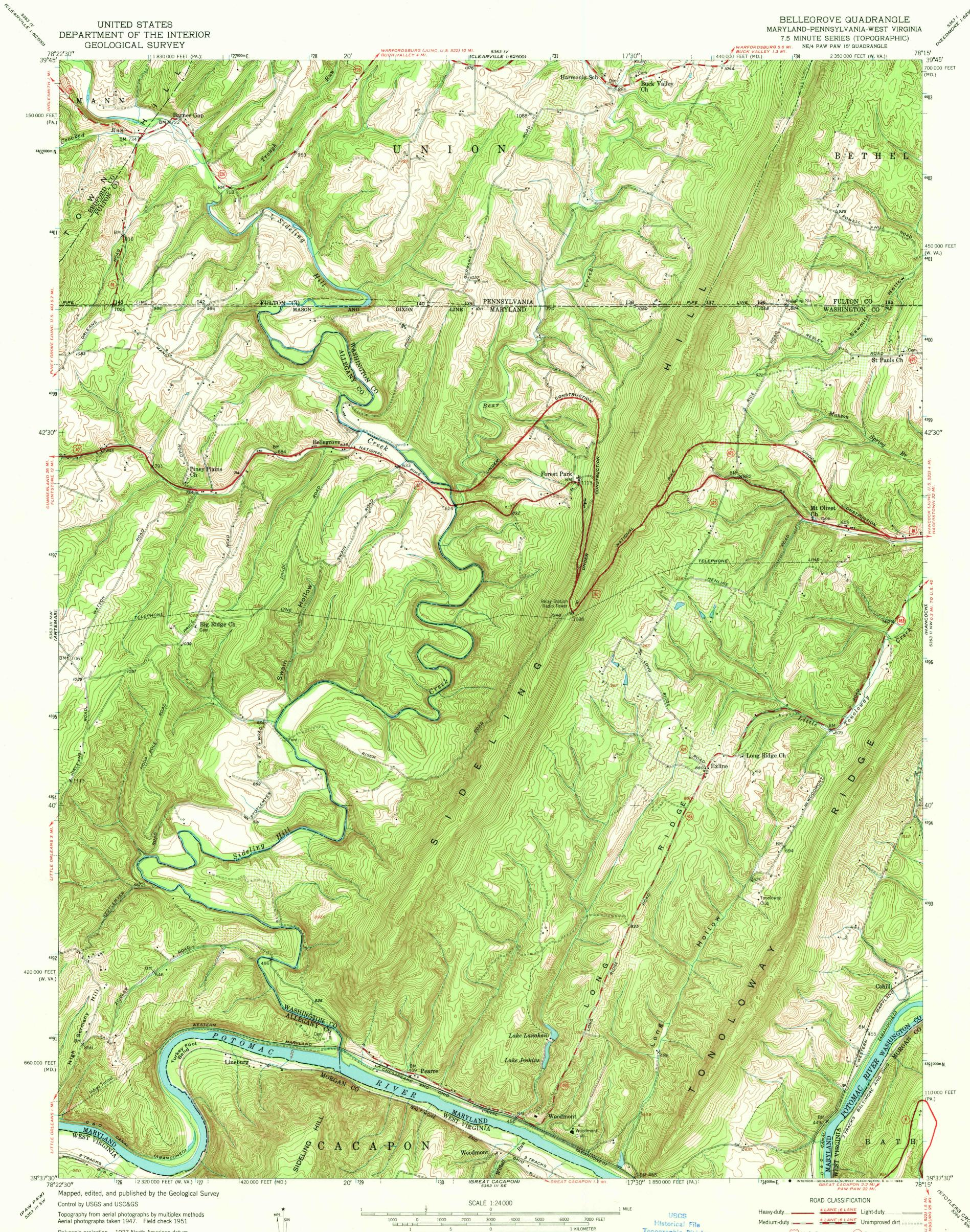
Polyconic projection. 1927 North American datum 10,000-foot grids based on Maryland coordinate system, Pennsylvania coordinate system, south zone, and West Virginia coordinate system, north zone 1000-meter Universal Transverse Mercator grid ticks, zone 17, shown in blue
