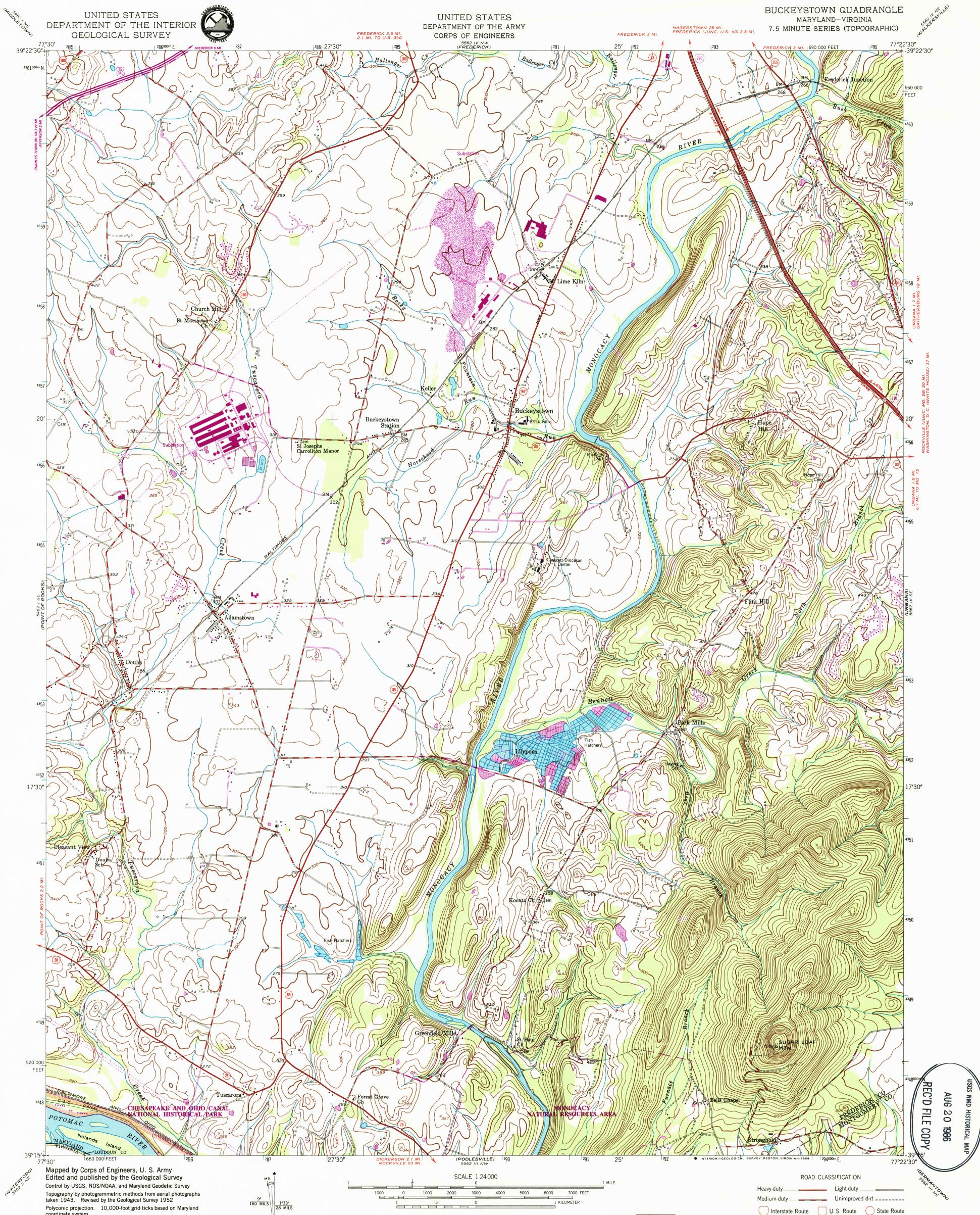
Polyconic projection. 10,000-foot grid ticks based on Maryland coordinate system 1000-meter Universal Transverse Mercator grid ticks, zone 18, shown in blue 1927 North American Datum To place on the predicted North American Datum 1983 move the projection lines 7 meters south and 25 meters west as shown by dashed corner ticks There may be private inholdings within the boundaries of the National or State reservations shown on this map
