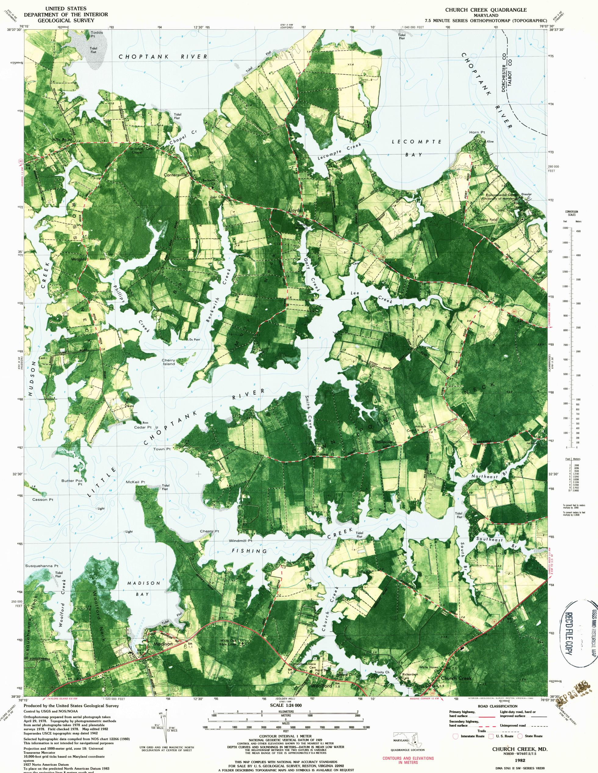
To place on the predicted North American Datum 1983 move the projection lines 8 meters south and 29 meters west as shown by dashed corner ticks
