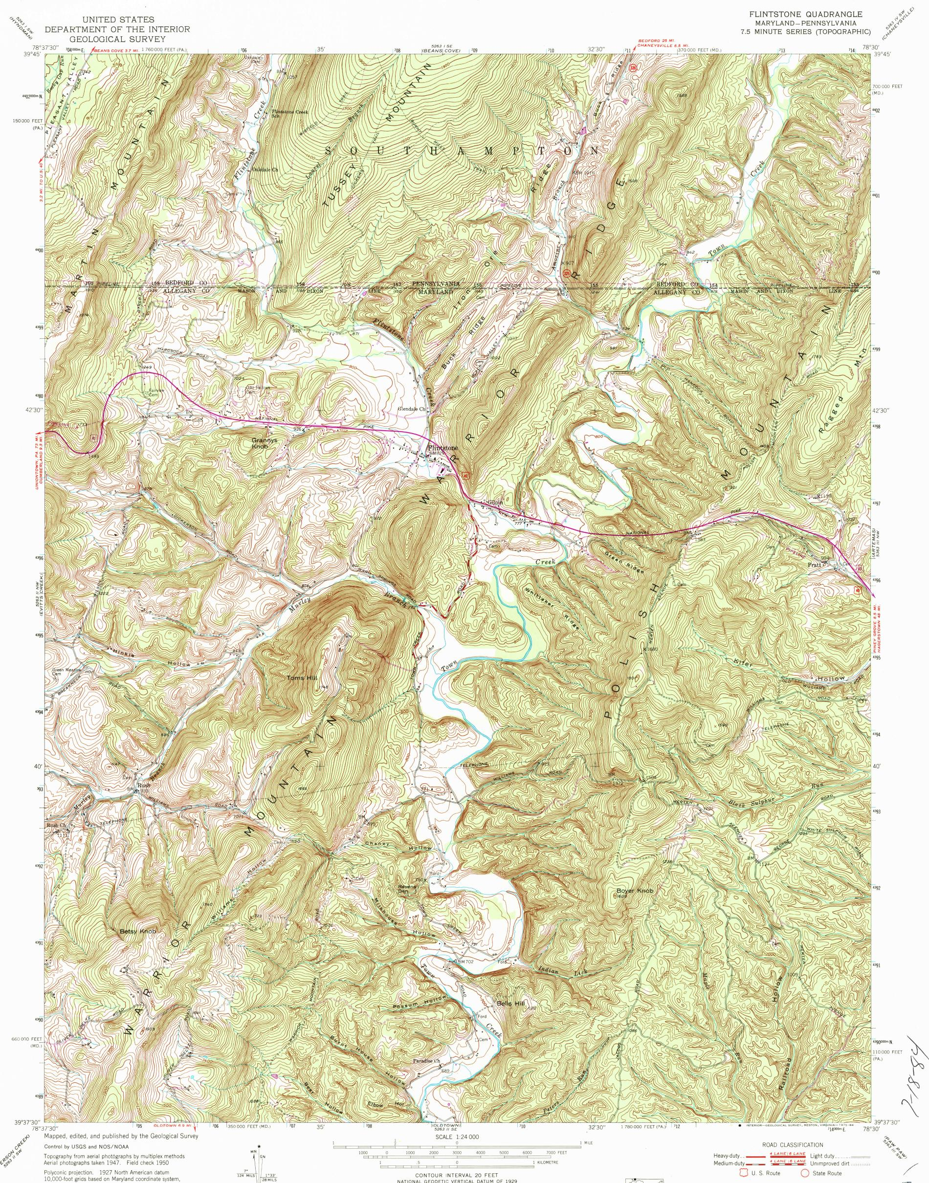
Polyconic projection. 1927 North American datum 10,000-foot grids based on Maryland coordinate system, and Pennsylvania coordinate system, south zone 1000-metre Universal Transverse Mercator grid ticks, zone 17, shown in blue
