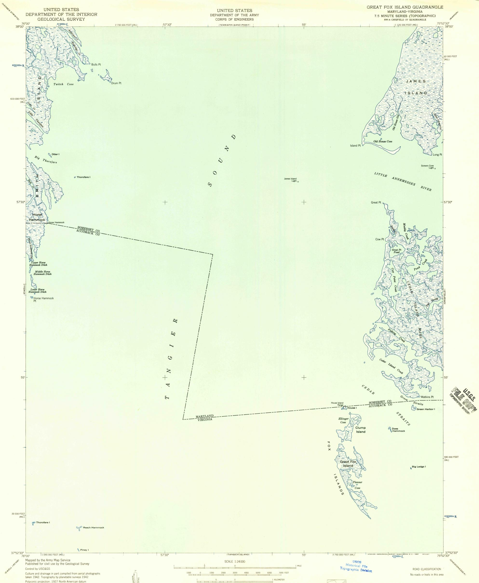
Polyconic projection. 1927 North American datum 10,000-foot grids based on Maryland coordinate system and Virginia coordinate system, south zone 1000-meter Universal Transverse Mercator grid ticks, zone 18, shown in blue
