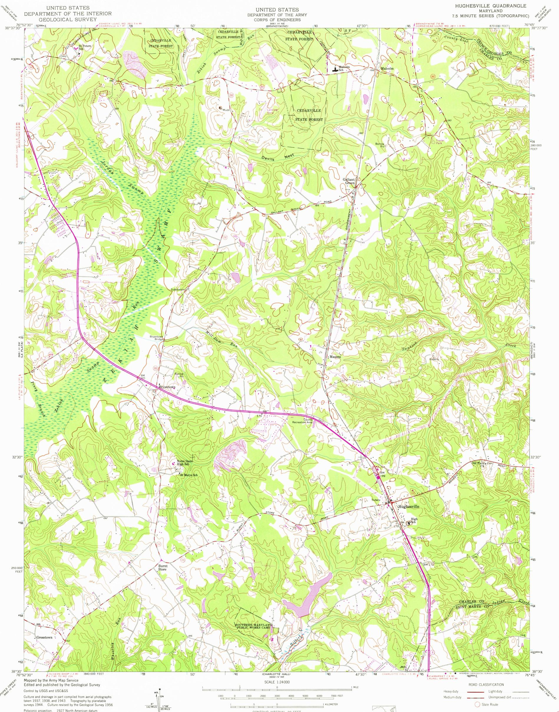
surveys 1944. Culture revised by the Geological Survey 1956 Polyconic projection. 1927 North American datum 10,000-foot grid based on Maryland coordinate system 1000-meter Universal Transverse Mercator grid ticks, zone 18, shown in blue Unchecked elevations are shown in brown
