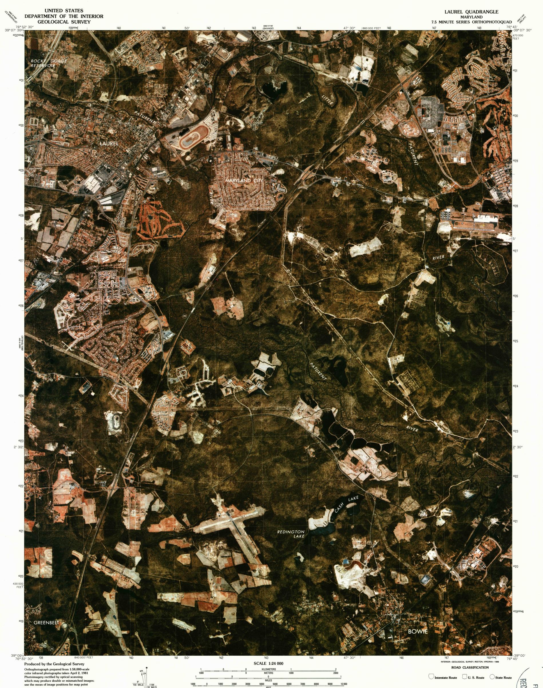
Projection and 1000-meter grid: Universal Transverse Mercator, zone 18 10,000-foot grid ticks based on Maryland coordinate system 1927 North American Datum To place on the predicted North American Datum 1983 move the projection lines 8 meters south and 27 meters west as shown by dashed corner ticks
